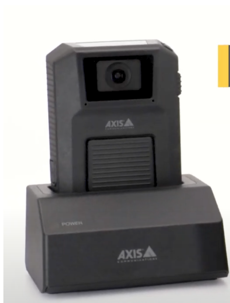
Figure 2.2: The BWC Docking station with a BWC in it
