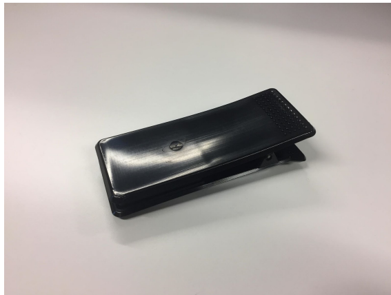
Figure 4.3: The clip attachment used for some recordings. When used, the clip attachment is attached to the clothes of the participant together with the BWC.
