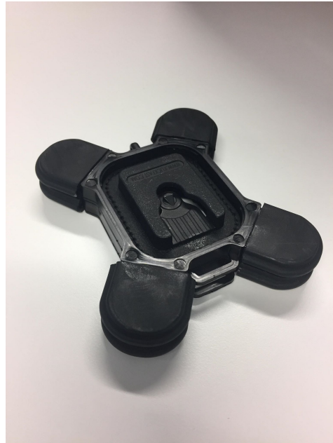
Figure 4.4: The magnet attachment used for some recordings. When used, the magnet attachment is attached to the clothes of the participant together with the BWC.
