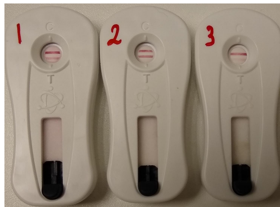
Figure 14 – The results from the Veriflow method. The cassettes are marked with number, where 1 indicates the smoothie sample, 2 apple concentrate and 3 apple beverage. The second cassette shows the strongest positive result, then the first, then the third with a weak positive.
