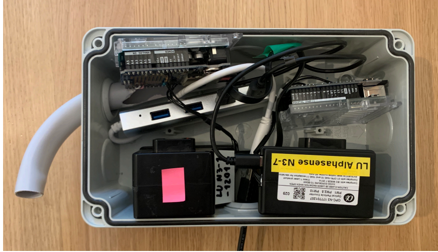
Figure 14: Two OPC-N3 sensors connected to Arduinos and data logging shields inside the plastic casing.
