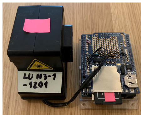
Figure 1: OPC-N3 wired to the Arduino and data logger shield.
