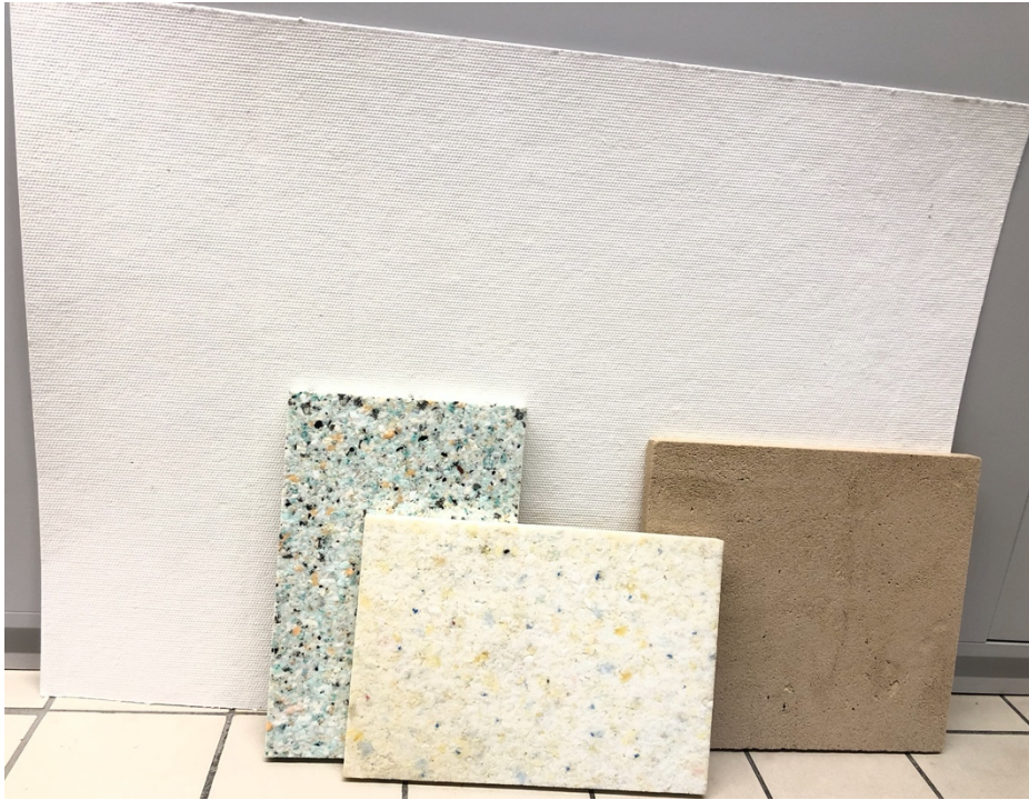
Figure 6.2 The materials picked for further development. From left to right: Circulose, Bonded Foam (two colors represented in picture) and Wood Foam.
