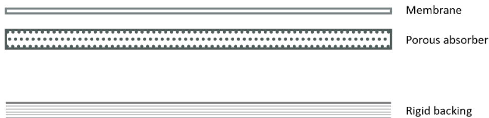
Figure 4.4 Helmholtz absorber and Membrane absorber
