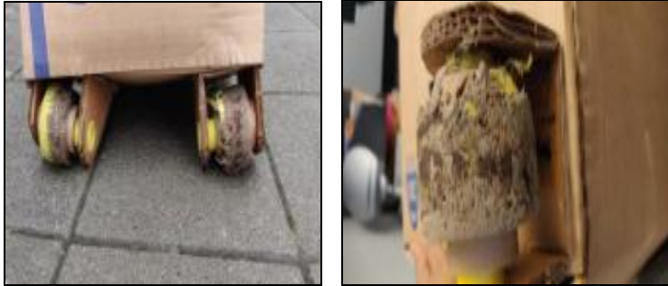
d) Wheels got damaged at 1.8 km
