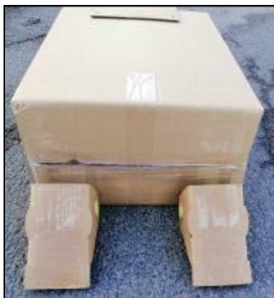
c) Failure at 1.5 km
