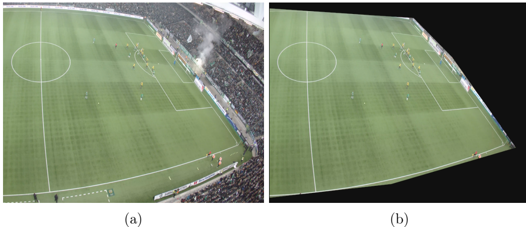
Figure 4.5: Example of how a mask is used to remove unnecessary information from images.
