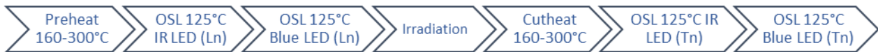
Fig. 4. Quartz standardized protocol, including preheat and cutheat temperatures determined before. This sequence is repeated for different doses.
