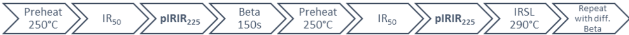
Fig. 6. The standardized feldspar protocol, the bold text shows the parts that are added by Buylaert et al. (2009). This set is repeated with three different Beta irradiations according to the feldspar dose, followed by the recuperation and at last the recycle regenerated dose.
