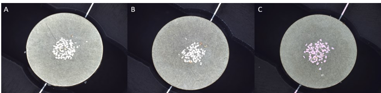
Fig. 13. Three aliquots on discs from different samples (A) 102 (B) 95 (C) 100 with an average of approximately 70 grains.
