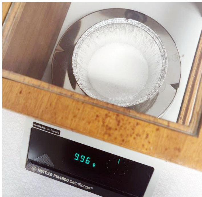
Figur 12. Torrt polymergranulat vägs in i aluminiumform.
