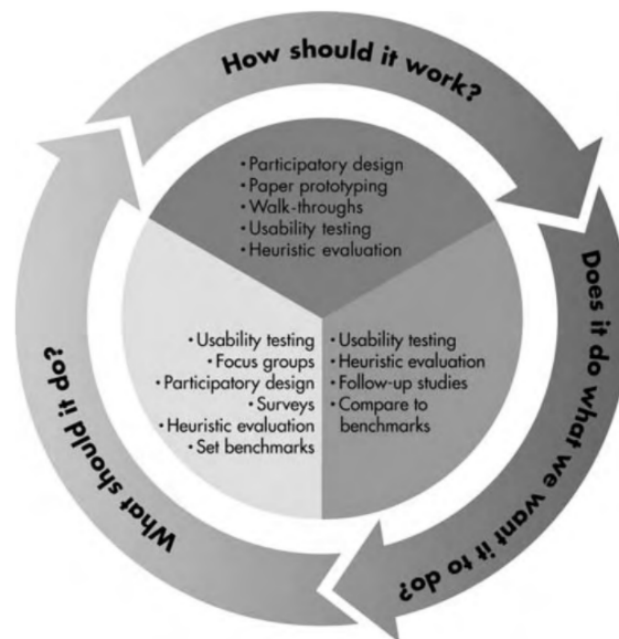
Figure 2.1: Questions and methods of answering them in an iterative design process. Rubin, J., Chisnell, D., 2008. Handbook of Usability Testing p.15
