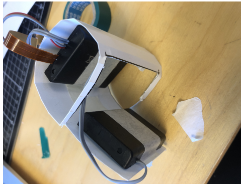
Figure 100: Battery placement on the hatch and inside.
