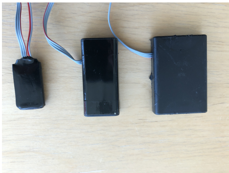
Figure 90: Three sizes of batteries.
