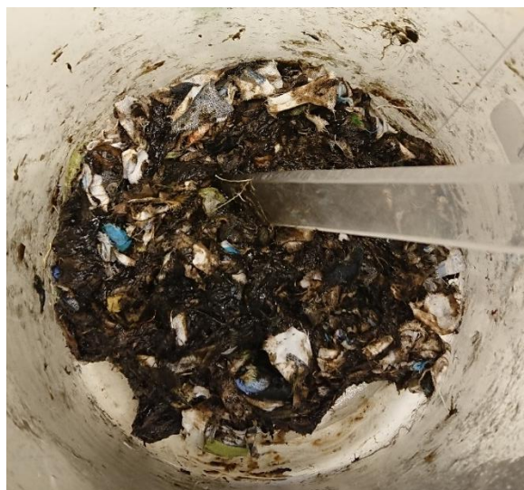
Figure 11. A mixture of dissolved, partially dissolved and undissolved textiles in 80% sulfuric acid.
