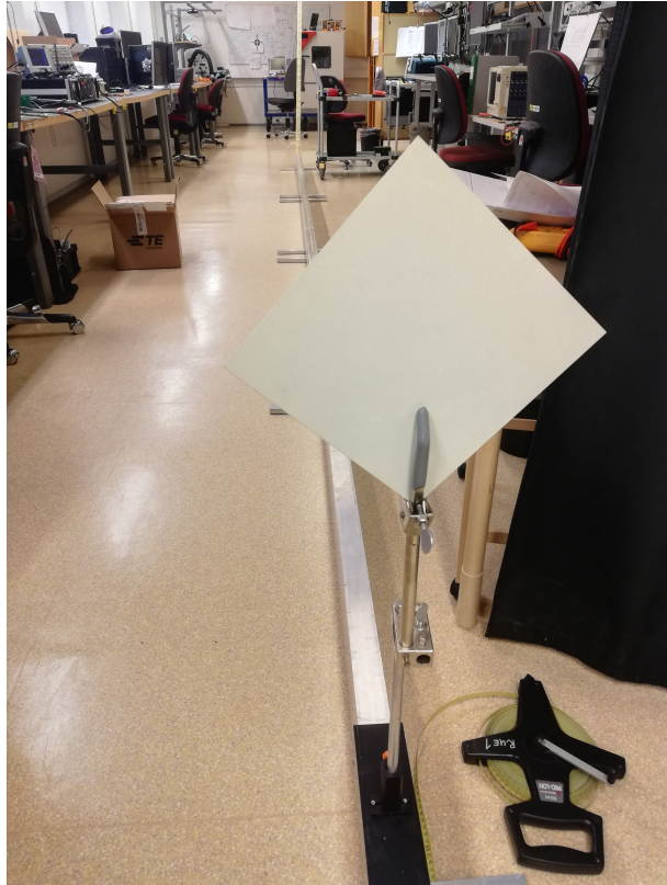
Figure 15: The figure shows the rail with holder for the targets. The rail was placed such that distances between 2.5-10 m could be measured. The first distance that where measured where 2.5 m. One measurement where taken for every plate and then the holder was moved 0.5 m further away from the LiDAR and new measurements where taken.
