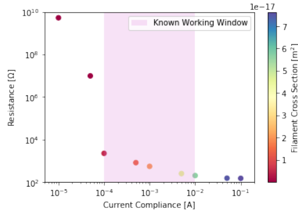
Figure 4.6: A visualisation of how LRS resistance R_{LRS} and filament cross section S behave as a function of parameter analyser current compliance.
