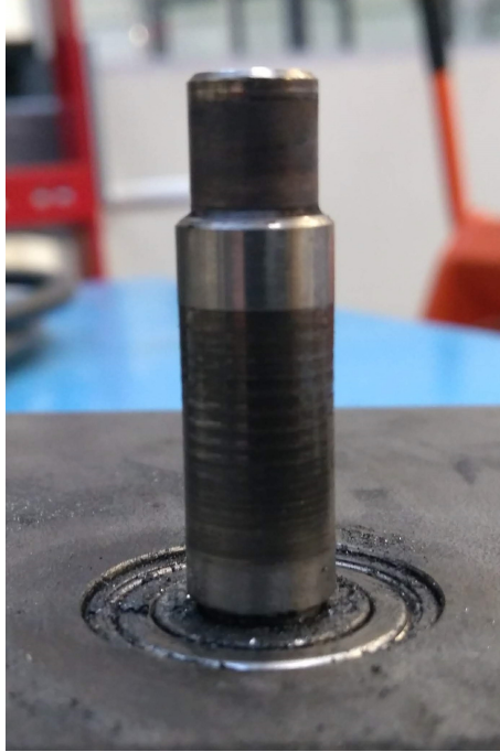
Figure 3.3: Image of wear patterns on the driving shaft resulting from cyclic loading in the test rig.
