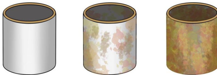
Figure 7.2 Concept illustration of the biodegradation of the PHB surface treatment with enzymes on a fibre-based drinking device.
