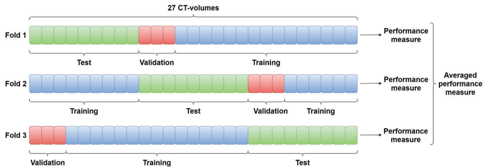
Fig. 17: This figure shows the partitioning of the 27 CT-volumes in the public dataset for the different folds in the 3-fold cross validation as well as the pipeline for obtaining the performance measure averaged across folds.
