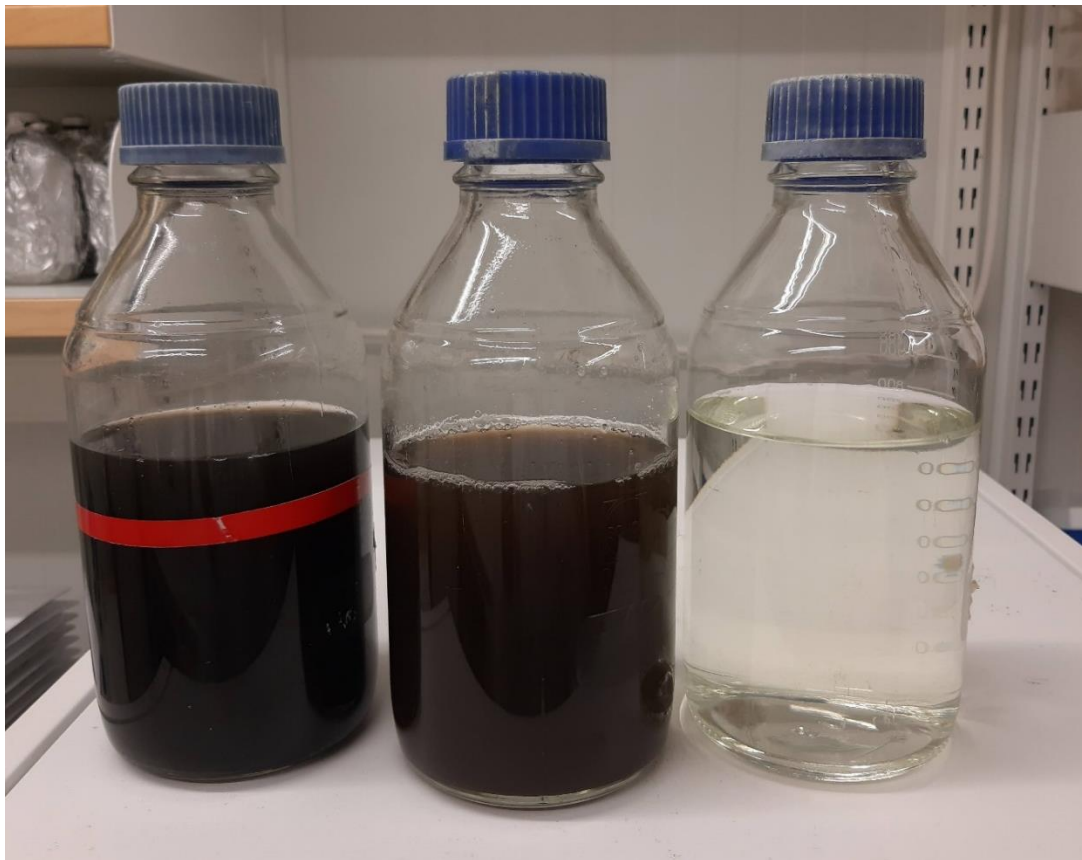
Figure 11. The three types of fertilizer investigated in this master thesis project. From left to right: Non-nitrified biofertilizer, nitrified biofertilizer, and inorganic fertilizer. (Photograph by J. Södergren, 2020)
