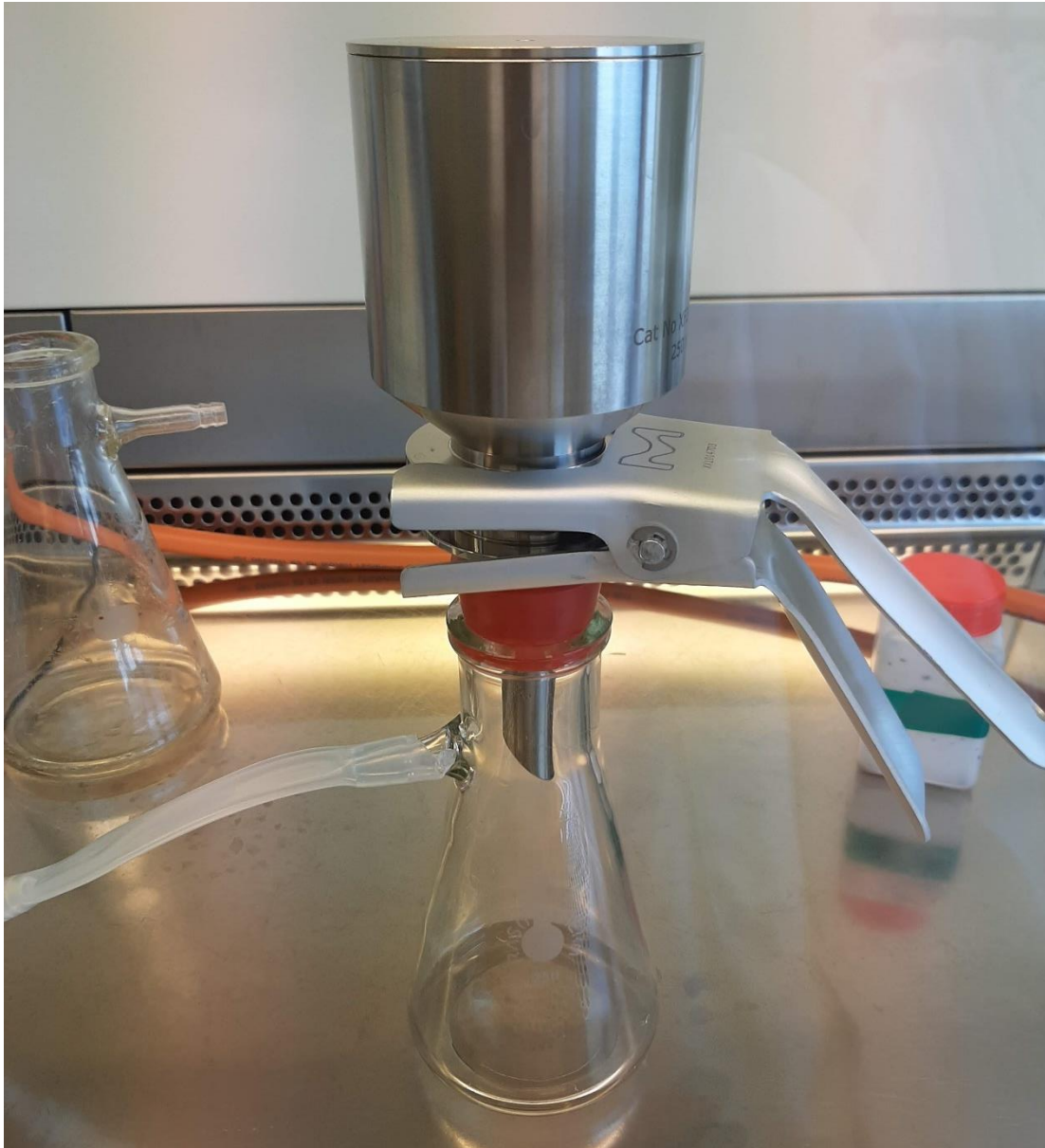
Figure 8. Filtration setup. Stainless steel funnel and filter holder held together with a clamp, inserted into a sidearm flask connected to a tube creating a vacuum. (Photograph by J. Södergren, 2020)
