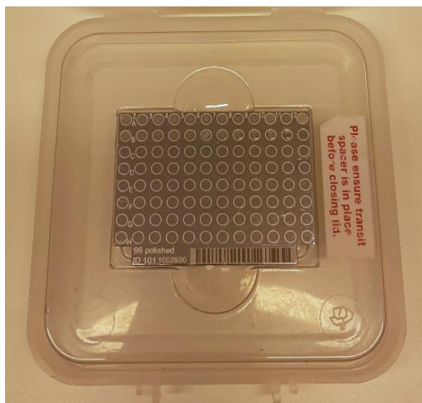
Figure 6. Target plate for MALDI-TOF Biotyping. Extract of a lysed colony is placed in a sample position (circle) on the plate, and the sample is fixed on the tablet with formic acid. The plate is then ready to be subjected to analysis in the MALDI Biotyper® (Bruker) instrument.
