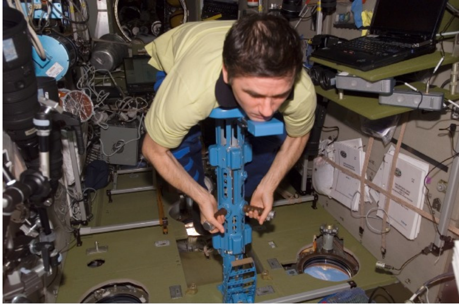
Figure 5: A cosmonaut measuring his body mass by holding onto a spring and measuring the frequency with which he oscillates. Photo: NASA
