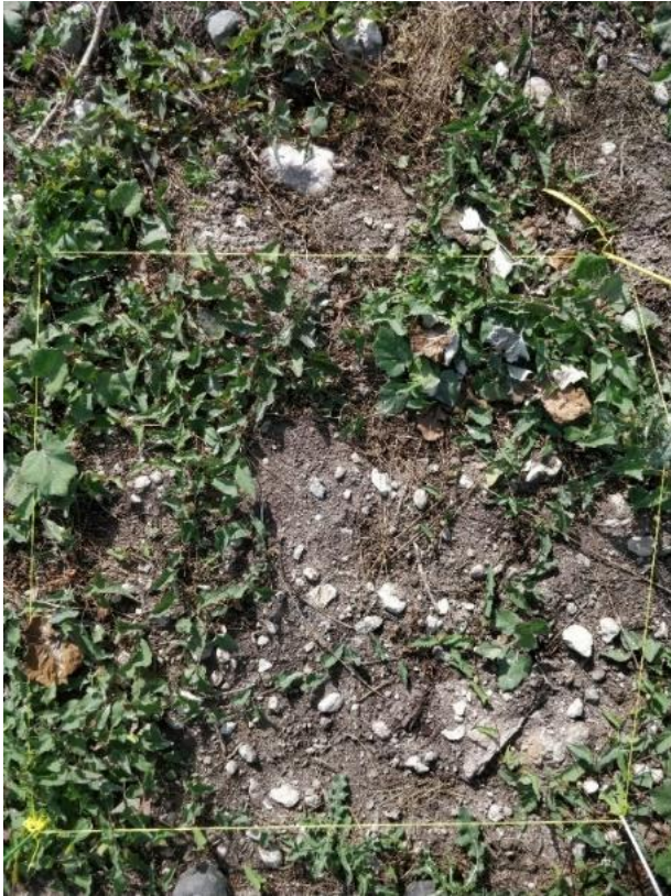
Figure 5. Monitoring quadrat used at the project site. Fiberglass rods mark out the corners of the quadrat and the frame is made out of a 2mm yellow cord.
