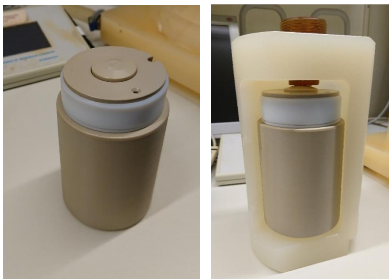
Figure 6. TFM microwave vessel with lid and safety spring in the HTC protection shield. To the right, the vessel is placed in the holder.
