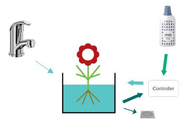
The picture above shows how an automatic controller was used to keep the nutrient mix fresh by adding a little bit of nutrient concentrate at a time. The plants absorbed the added nutrients as they grew, and the levels automatically remained in range, without manual work. The controller used simple and low-cost electronics to measure the electrical resistance of the water. Since nutrients in water are dissolved ions, they conduct electricity, making this possible.
