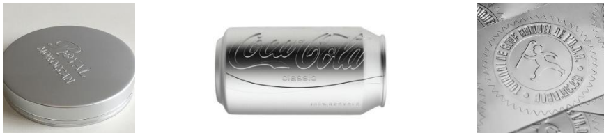
Figure 31: Embossing examples: Embossing of text, embossed can and embossing of logo (Alibaba, 2020; Kozak, 2019; Yoon & Lee, 2009)
