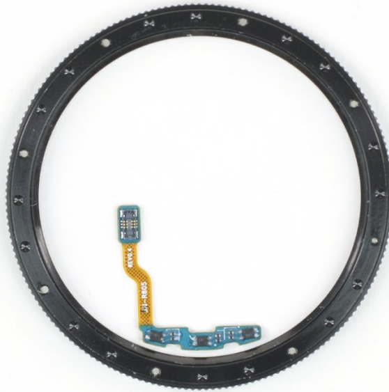
Figure 3.13: The rotating bezel of the Samsung Galaxy Watch. [24]
