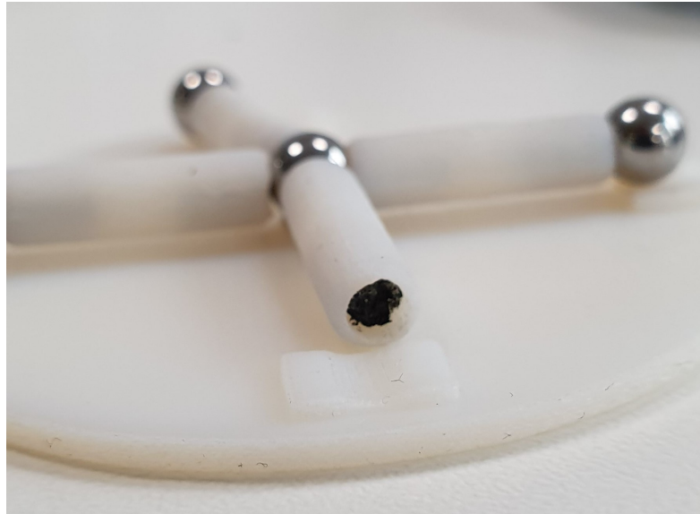
Figure 6.12: A small amount of foam was inserted into the bores of the sticks in order to keep the magnets in place.
