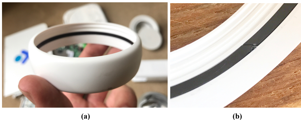
Figure 3.16: a) The magnetic strip used in the outer ring. b) Flat strip rolled up and adhered to the inside of the ring. [26]
