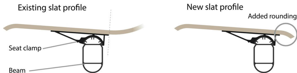
Figure 6.3: Illustration of the seat attached to the beam.
