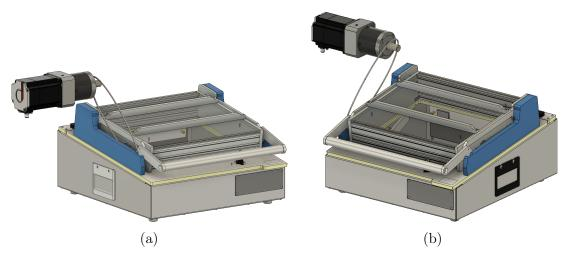
Figure 2.3: A rough illustration of how a chain could be fastened to a servo to automatically open and close the FCT-fixture.
