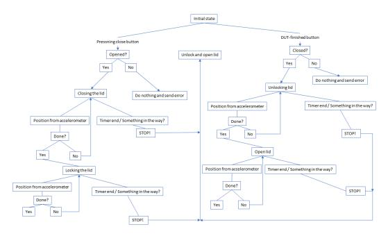
Figure 2.7: Flowchart over how the code should be generally implemented.
