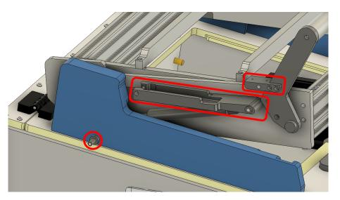
Figure 2.16: All cylinder fastening parts mounted to the FCT-fixture. The parts are circled in red.
