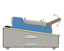
(a) This motion will be called locking or unlocking depending on the direction of the lid.
