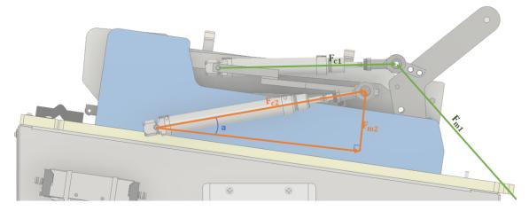
Figure 2.9: Illustration and notation for force calculations.  $F_{m1}$  is perpendicular to the handle.
