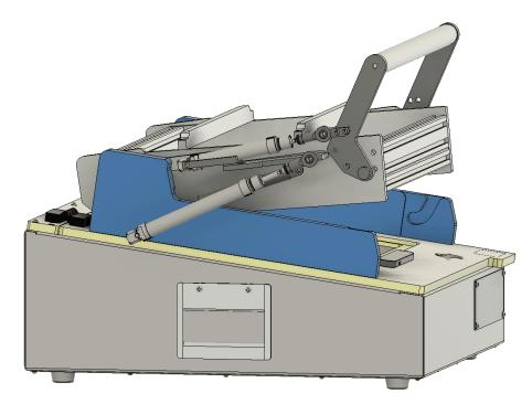
Figure 2.2: Illustration of how pneumatic cylinders could be fastened to automatically open and close the FCT-fixture.
