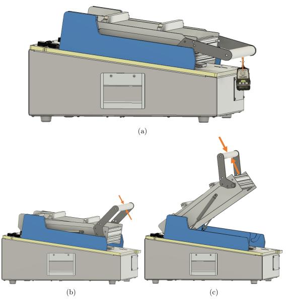
Figure 2.8: The orange arrows show how the force gauge was pushed to measure the forces. Figure 2.8a also shows a picture of the force gauge.
