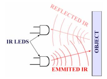
Figure 2.5: A simple illustration of how an IR proximity sensor works [7]. "OB-JECT" is fingers, hands or arms in this case.
