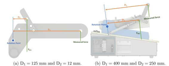
Figure 2.10: The forces measured
