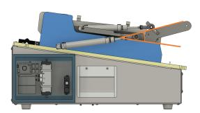
(a) The angle shown in the figure is the angle measured from fully locked to closed but not locked.
