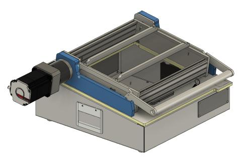
Figure 2.1: Illustration of how a servo could be placed to open and close the FCT-fixture.
