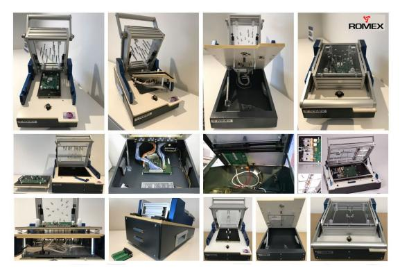
Figure 1.1: Several pictures of a FCT-fixture by MG modified by Romex. The needles are visible in the bottom left picture [6].
