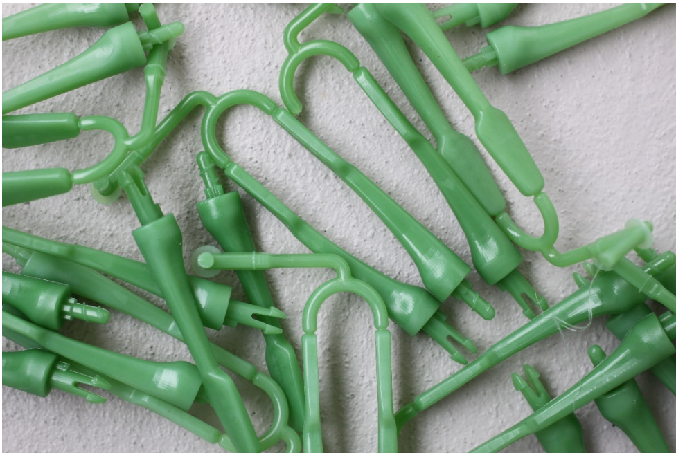
Figure 87. Selection of injection moulded prototypes before separation.
