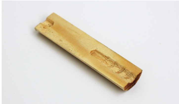
Figure 71. Threaded mark in pinewood using the aluminium threaded pin.
