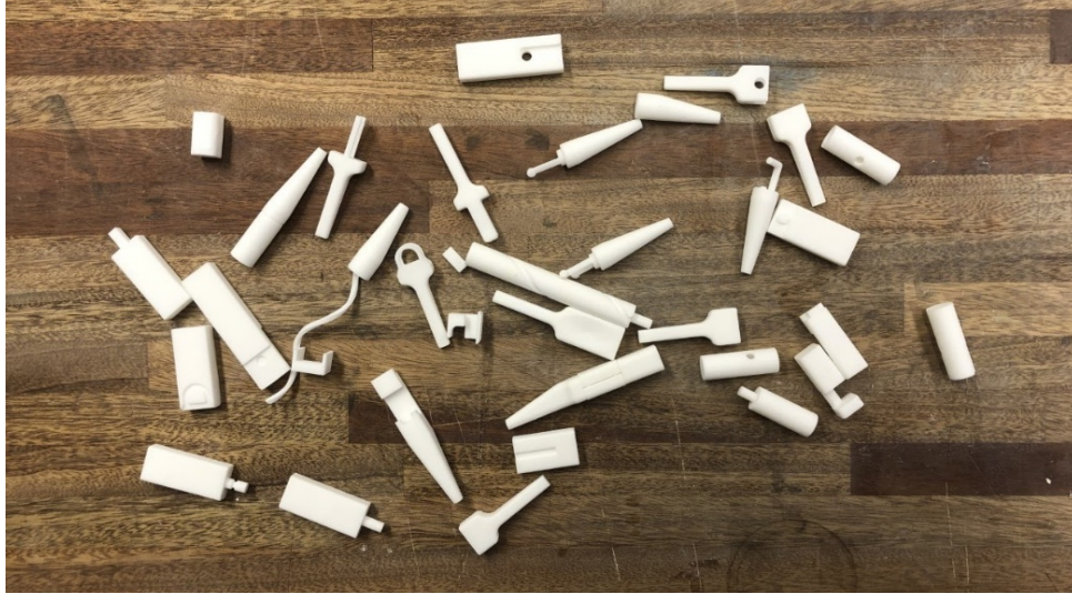
Figure 24. Picture of the 3D printed models in PA using the SLS method.
