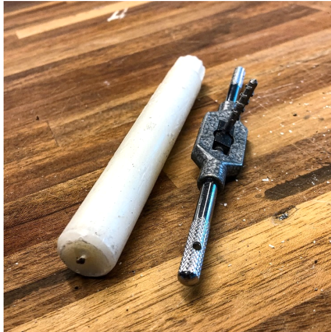
Figure 74. Threaded pin and tap wrench used to thread the hole.
