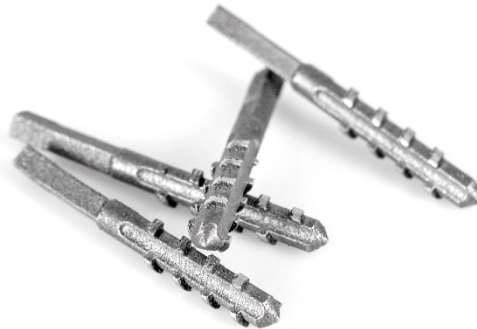
Figure 70. The 3D printed threaded pins in aluminium.
