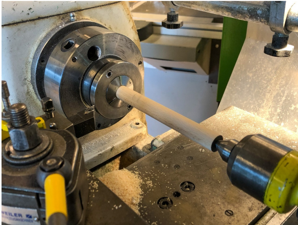
Figure 77. Dowel fastened in the lathe before turning it to the accurate diameter and polishing the surface.
