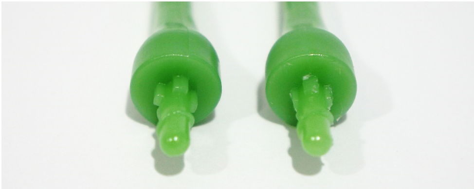
Figure 54. Picture of the original plastic ribs to the left and the modified to the right.
