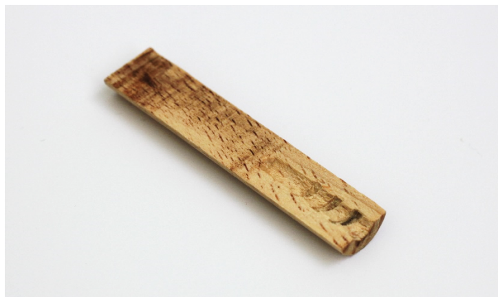
Figure 72. Threaded mark in beech using the aluminium threaded pin.
