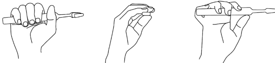
Figure 15. Most common grips. Whole hand grip to the left, finger grip in the middle and high edge grip to the right.
