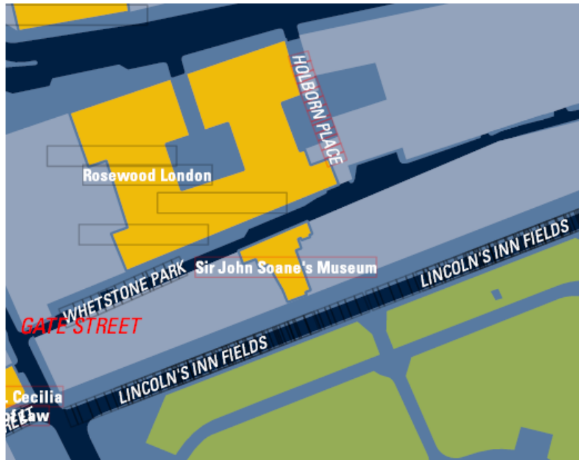
Figure 4.4: Example of polygon and line feature label placement using the Automated Placement Engine. Unplaced labels are in red. The candidate label positions are shown as boxes. Note that the road labels have a box for every character. This is because they are set to be curved. Straight (parallel) labels have one box per label. Based on data from © T-Kartor Group AB.
