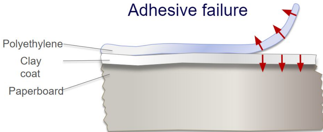
Figure 3: Adhesive failure. Note that the figure is not to scale.
