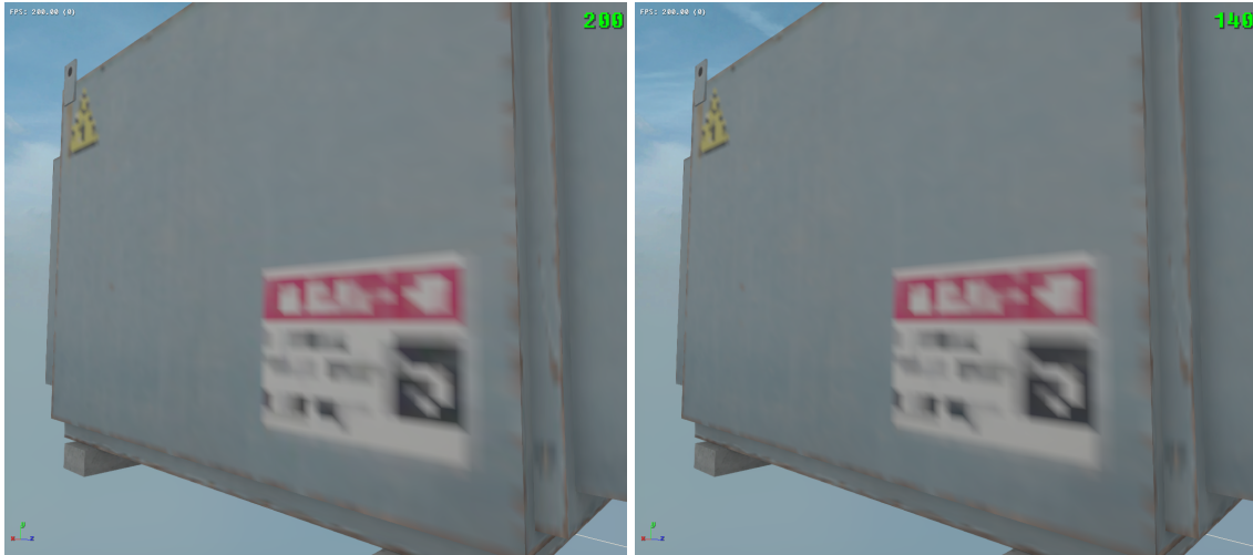
Figure 3.4: Rendering with MCC-compressed texture (left) and uncompressed texture (right). Faces in both models have a resolution of 64. Compression ratio: 6.4517.
