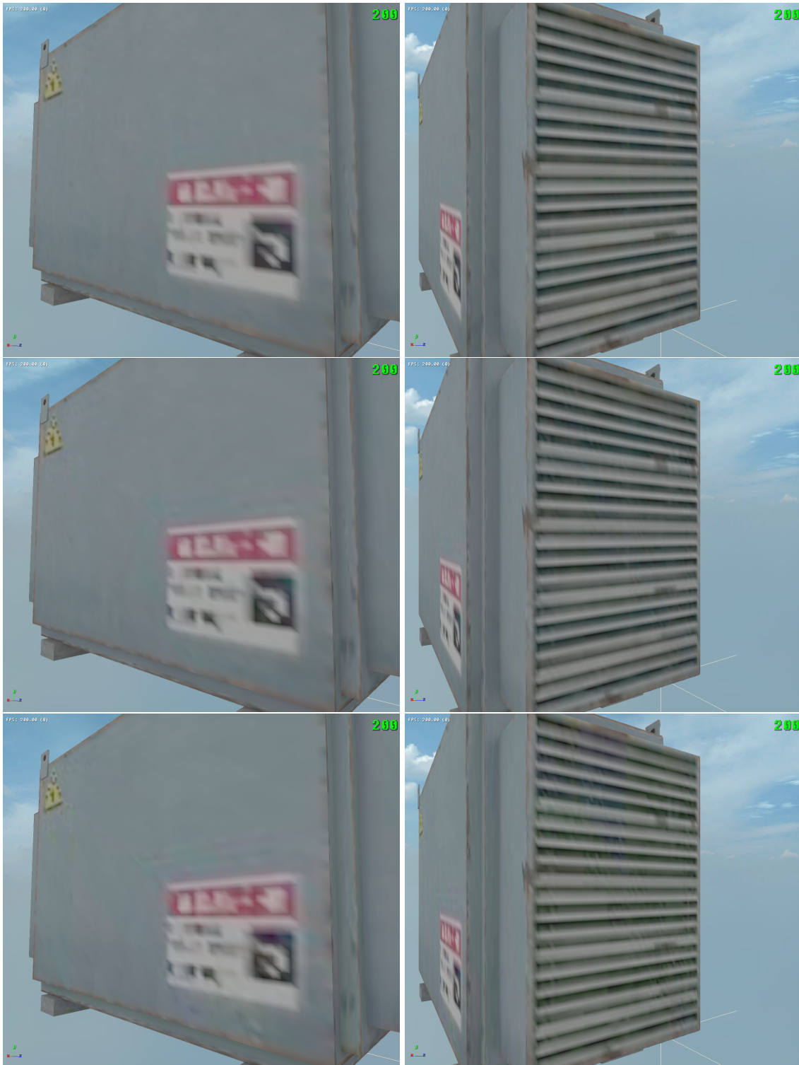
Figure 3.8: Renders of the model textured using mesh colors data with compression ratios of 12.00 (top), 17.87 (middle) and 27.74 (bottom).
