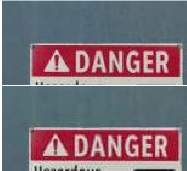
Figure 3.17: Ringing artifacts near an edge in the JPEG compressed source image. The images have a compression ratio of 21.7687 (top), and 39.0244 (bottom).
