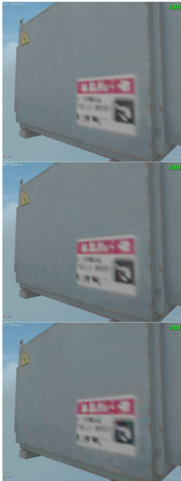
Figure 3.5: Rendering of model textured with decompressed mesh colors data with compression ratios of 9.54 (top), 14.62 (middle) and 23.43 (bottom).
