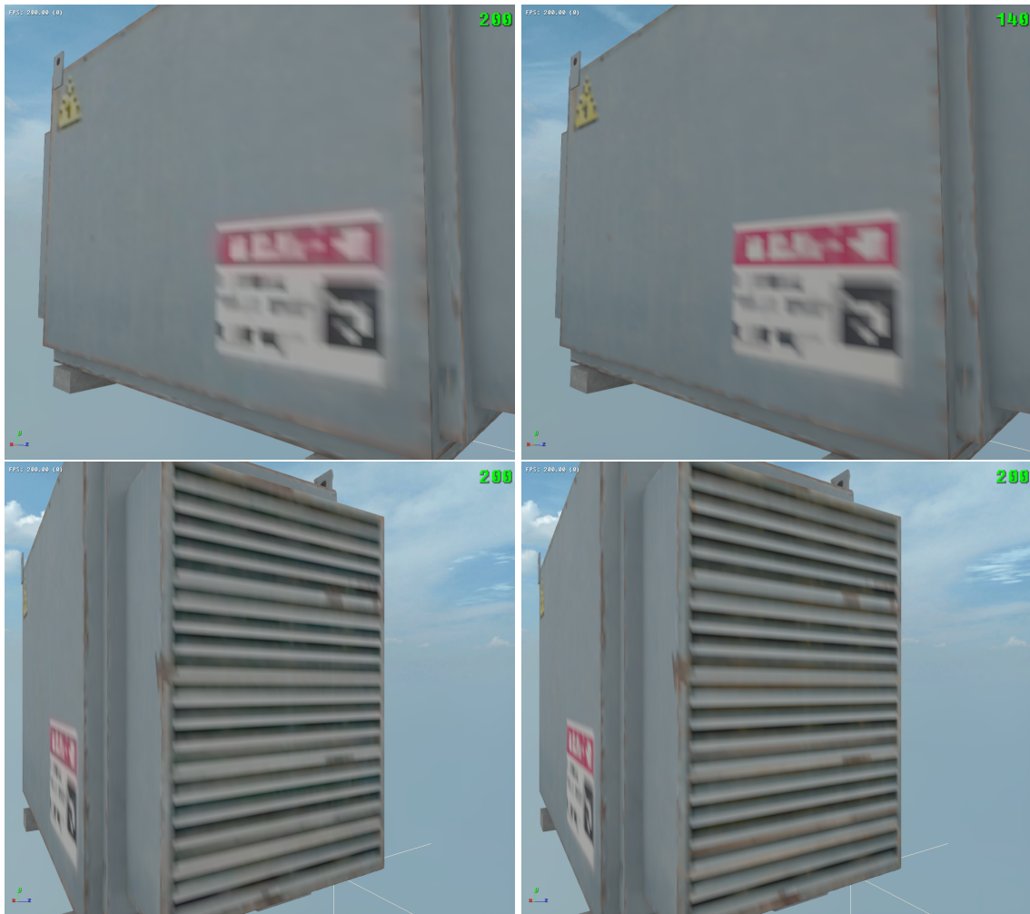
Figure 3.7: Renders with compressed mesh colors data (left-column) and uncompressed mesh colors data (right-column).
