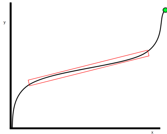
Figure 3.2: An illustration of how a non linear relation can be represented as a linear regression. As long our data is within the selected area, the relation seems linear. But if samples from the top right circle are included, our model gets thrown of.
