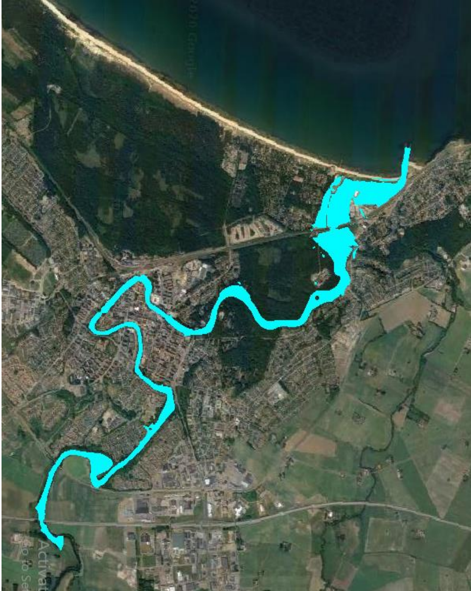
Figure 2.16: A flood map for 100-year flow from SMHI by the HEC RAS model
