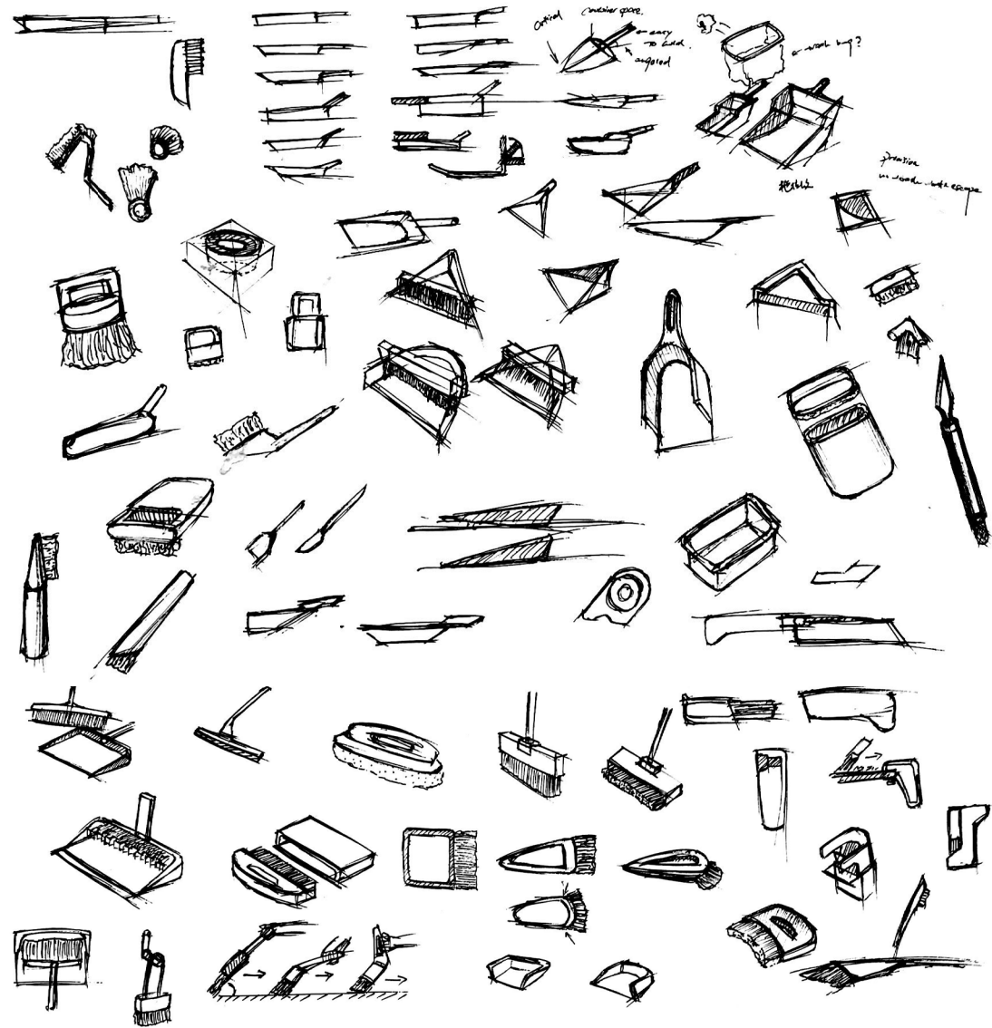
I tried to sketch different shapes of the cleaning parts and the scoop parts for my dustpan design
