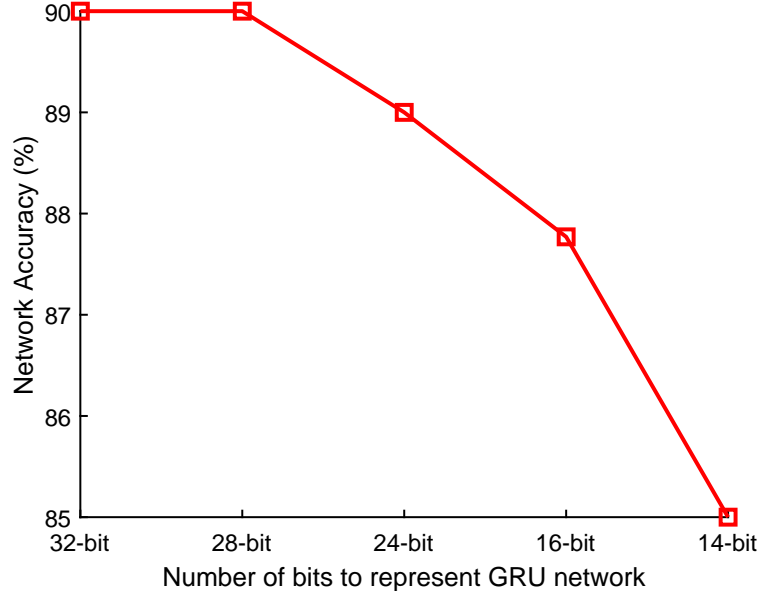
Figure 3.12: Network accuracy for GRU network with different precision bits to represent the network.
