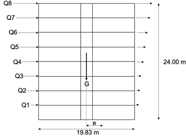
Figure F.2: Set-up of forces acting on the building when analysing the risk of tilting. Seen from short side of building.
