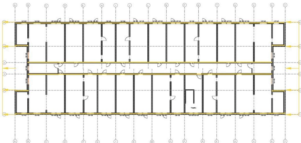
Figure A.10: Stabilising walls if wind load acts on the short side of the building.
