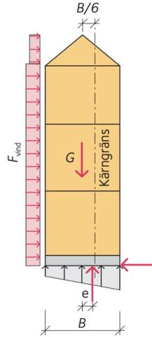
Figure 3.1: Control of overturn with the core boundary plotted. The illustration is from the CLT handbook, Svenskt trä (2015) and used with permission. (Kärngräns = Core boundary).
