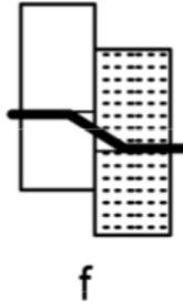
Figure 5.12: Failure mode (f) (EC5-1-1, 2009). Used with permission.
