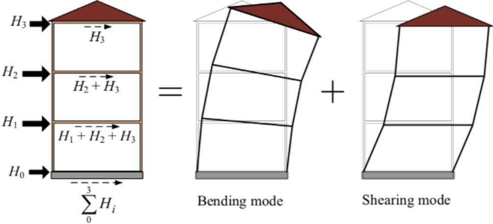
Figure 3.9: The distribution of the horizontal loads and bending and shear deformation for the floor levels of the building (Källsner & Girhammar, 2008). Used with permission.
