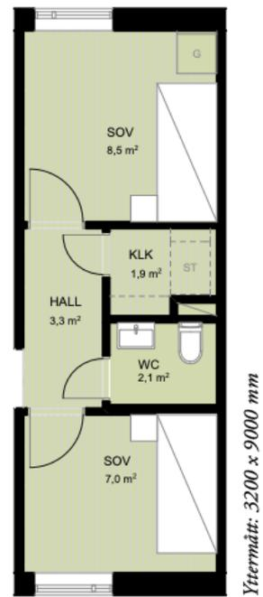
Figure A.3: Volume type 1, 2, 5 and 6. Translation: Yttermått=Outer dimensions and kvm=m<sup>2</sup>(Plusshus, 2017).
