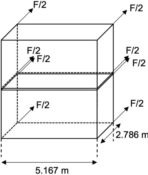
Figure F.5: The division of fasteners for the two top modules in wall B or wall X.
