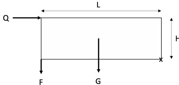
Figure 4.11: Set-up of forces acting on the uppermost module.
