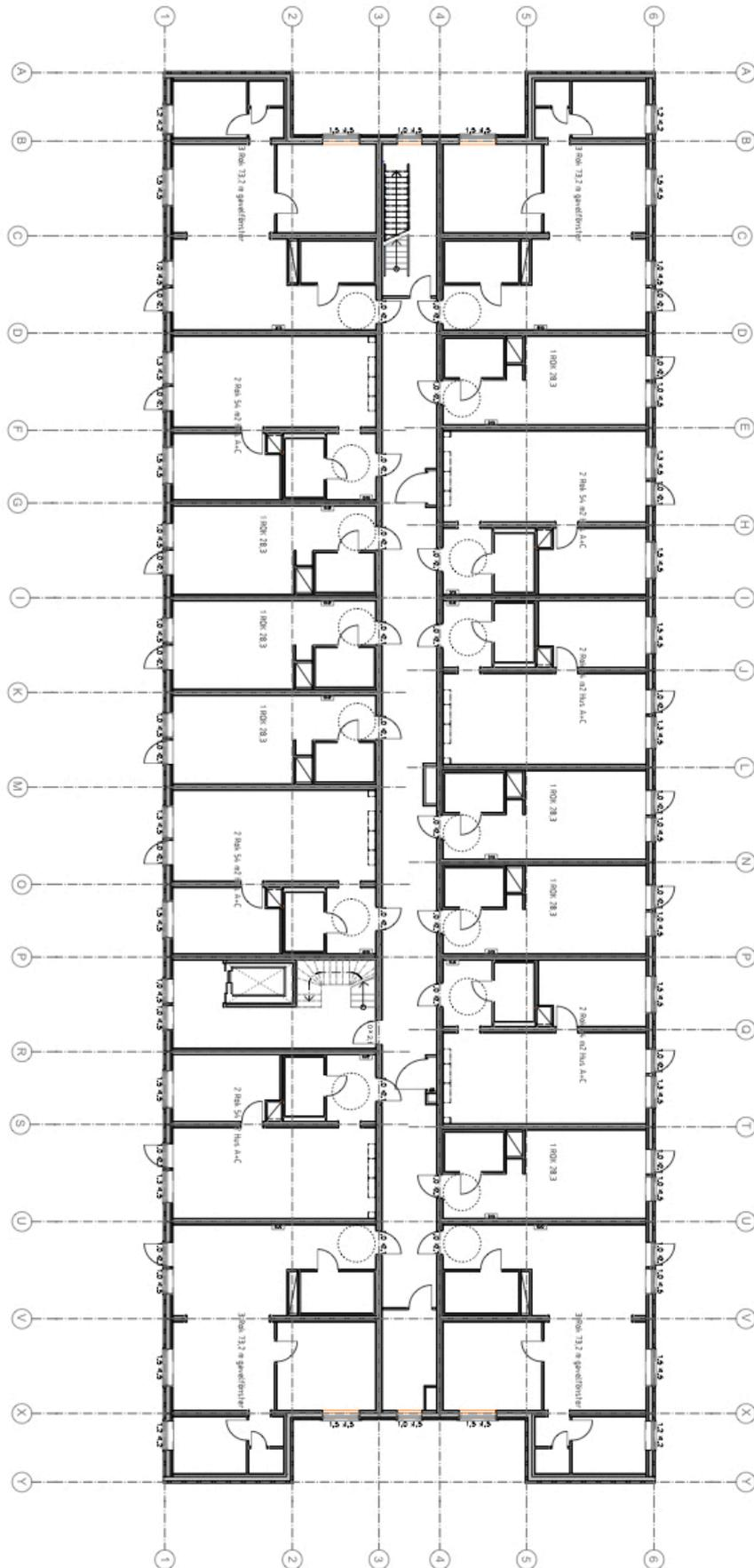
Figure A.15: Floor plan of the investigated building with naming of stabilising walls.
