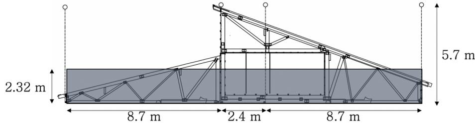
Figure F.4: Equivalent height of triangular area of influence.
