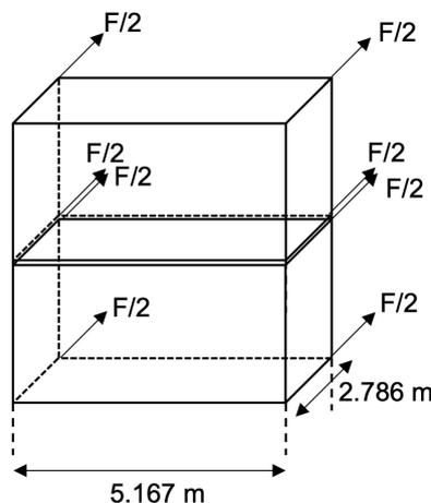
Figure 5.13: The distribution of the load for the fasteners holding the two top modules in wall B or wall X in place.
