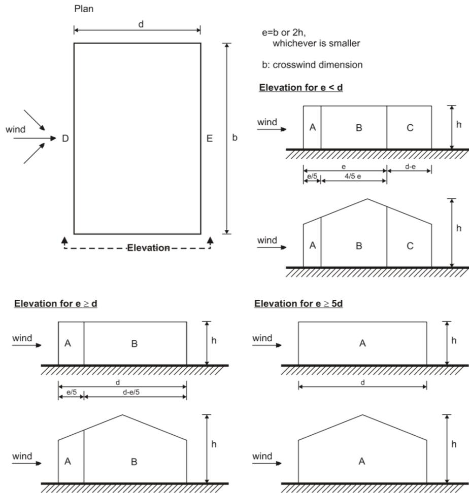
Figure B.2: Key for zone division and pressure coefficients for vertical walls (EC1-1-4, 2008). Used with permission.
