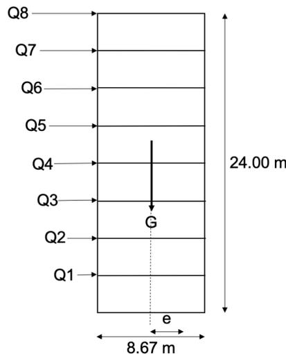
*Figure F.1: Set-up of forces acting on structure when analysing the risk of tilting. Seen from short side of building.*
