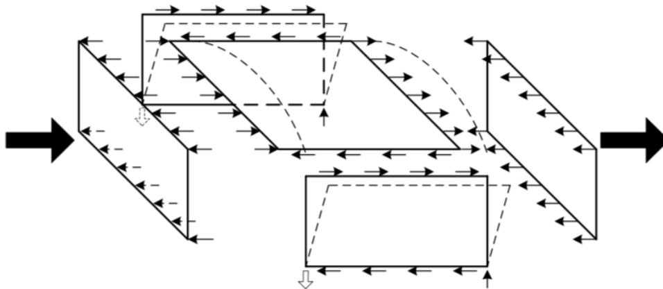
Figure 3.7: How the horizontal loads are carried by the walls and the floor structures to the ground (Källsner & Girhammar, 2008). Used with permission.
