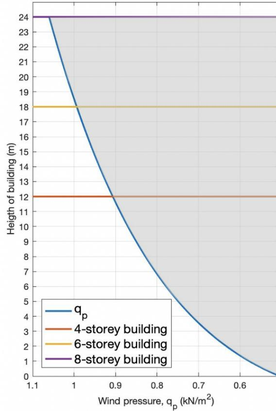
Figure B.6: Wind pressure for different heights. The three different storeys of buildings are marked. The grey area is the wind load.
