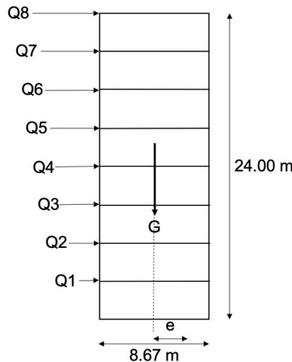
Figure 4.7: Set-up of forces acting on structure when analysing the risk of tilting. Seen from short side of building.
