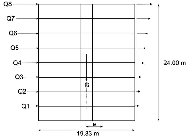
Figure 4.8: Set-up of forces acting on the building when analysing the risk of tilting for the whole building.
