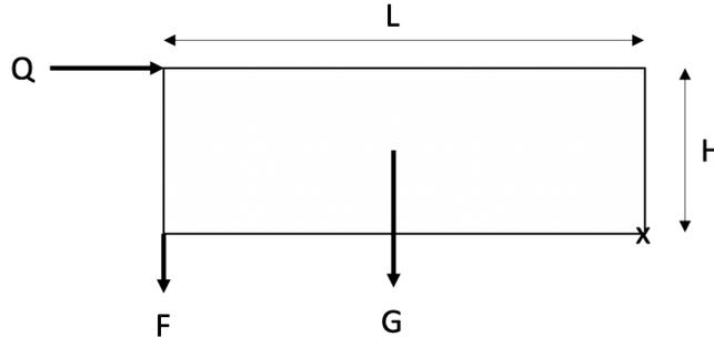
Figure 3.6: Evaluation of anchoring for top modules. View from the short side of the building.
