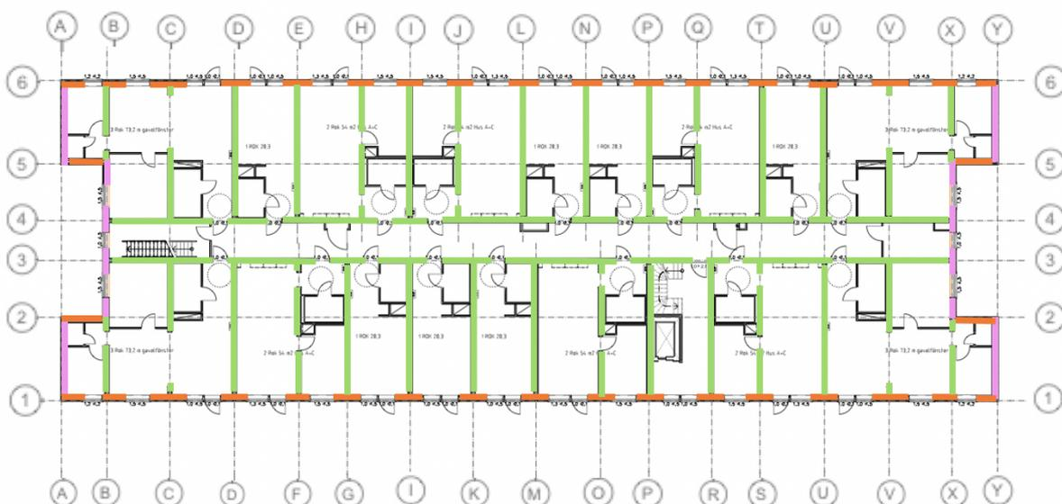
Figure A.14: The materials of the different walls. Orange = OSB, Pink = OSB and Fibre gypsum, Green = Fibre gypsum.
