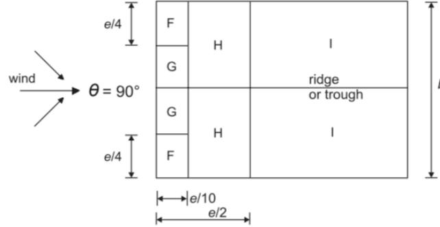
Figure C.2: The outspread of the different zones when the wind load is acting on the gable (EC1-1-4, 2008). Used with permission.
