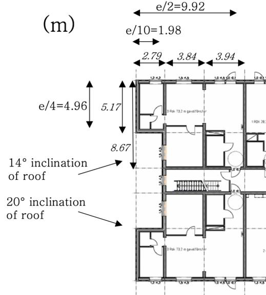
Figure 4.3: The three outermost modules which are analysed for uplifting forces.
