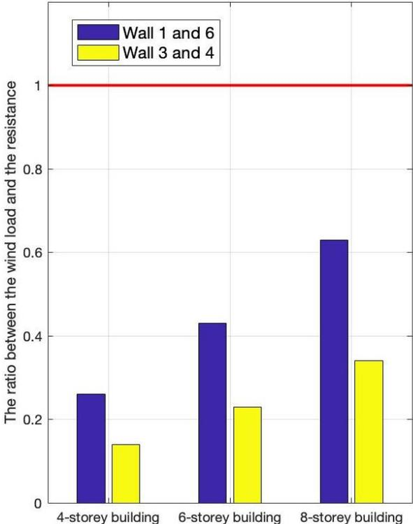
Figure 5.6: The ratio between wind load and the capacity according to Method A for the walls in the longitudinal direction of the building. Values lower than 1 indicates capacity > load. Wind on wall A or Y.
