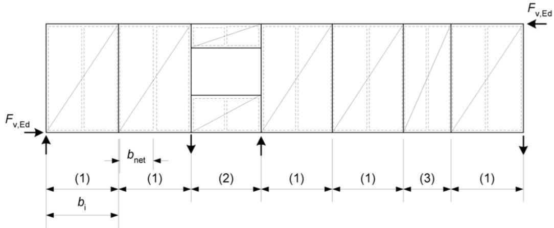
Figure 3.13: Wall segment consisting of several panels (EC5-1-1, 2009).
