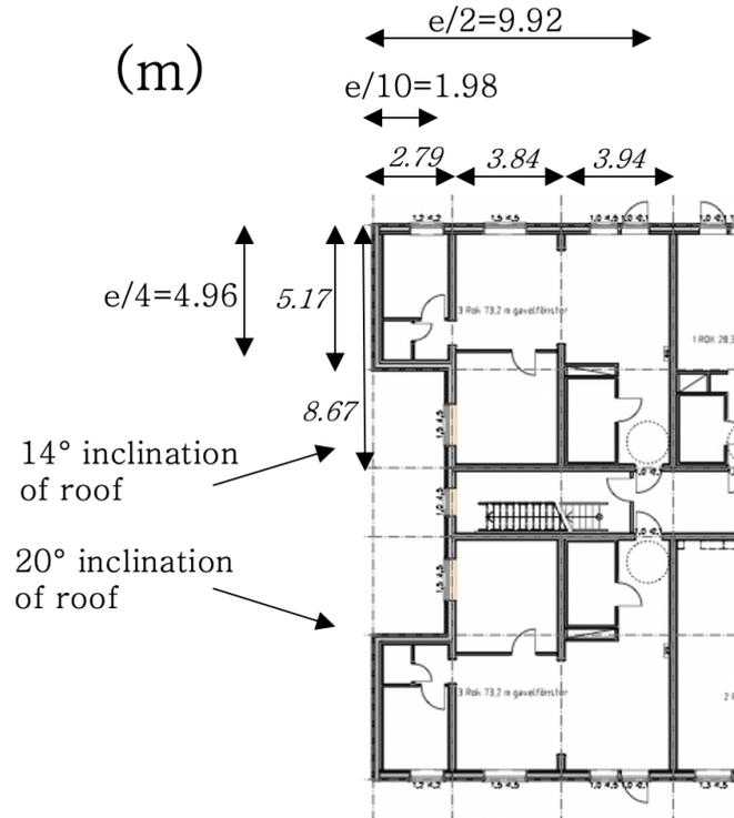
Figure C.3: The three outermost modules that are analysed for uplifting forces.
