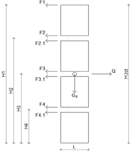
Figure 3.4: Evaluation of tilting according to Derome.
