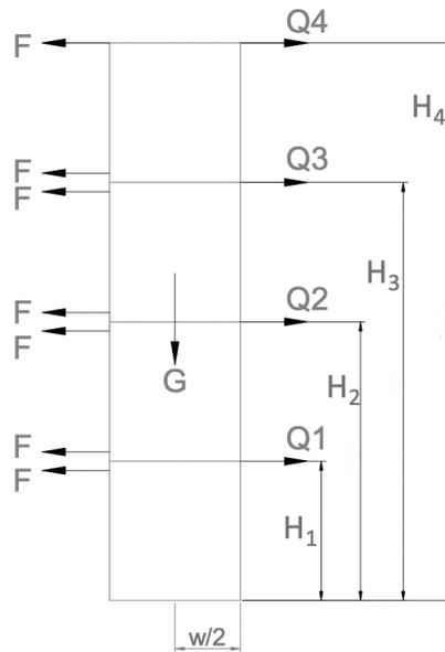
Figure 4.9: The forces of interest when analysing the need of anchoring of the outermost modules for a four-storey building.
