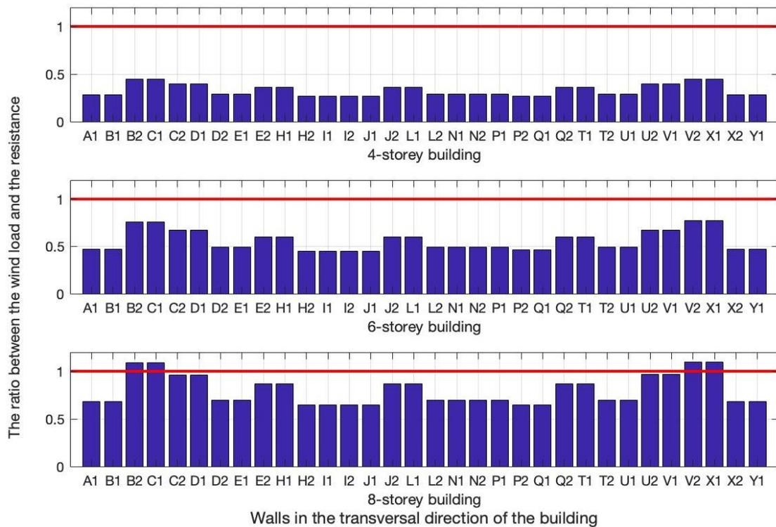
Figure 5.8: The ratio between the wind load and the capacity for all walls in the transverse direction of structure 2 for a 4-, 6- and 8-storey building. Values lower than 1 indicates capacity > load. Wind load on wall 6.
