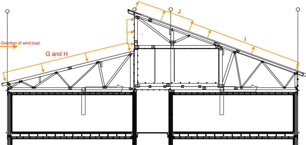
Figure B.8: Worst case for pressure coefficients when the wind load acts on wall 6.
