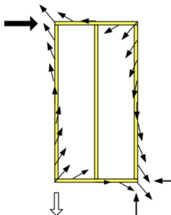
Figure 3.10: Force displacement for elastic calculation model (Källsner & Girhammar, 2008). Used with permission.
