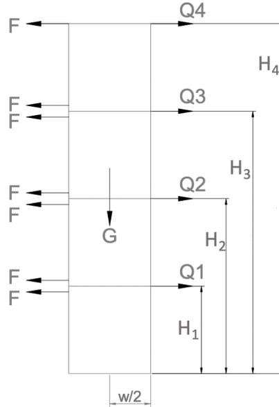
Figure F.3: Forces acting on the outermost modules.
