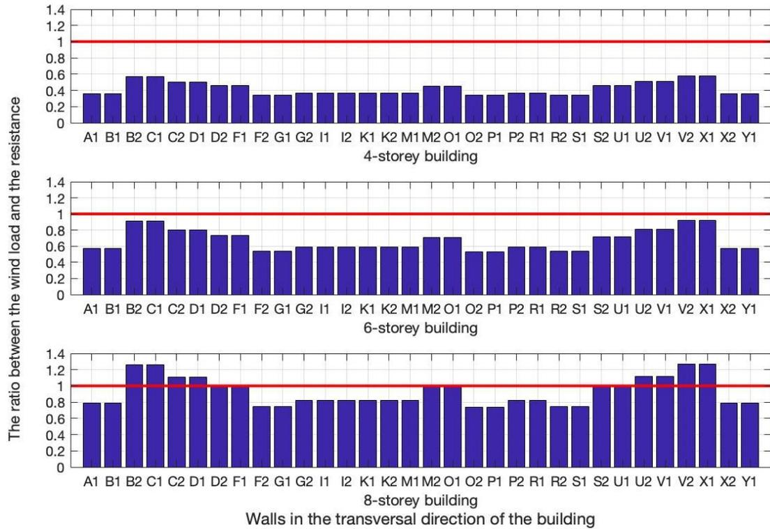
Figure 5.7: The ratio between the wind load and the capacity for all walls in the transverse direction of structure 1 for a 4-, 6- and 8-storey building. Values lower than 1 indicates capacity > load. Wind load on wall 1.
