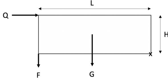
Figure F.6: Set-up of forces acting on the uppermost module.
