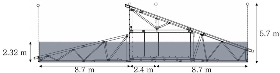
Figure 4.10: Equivalent height of triangular area of influence.
