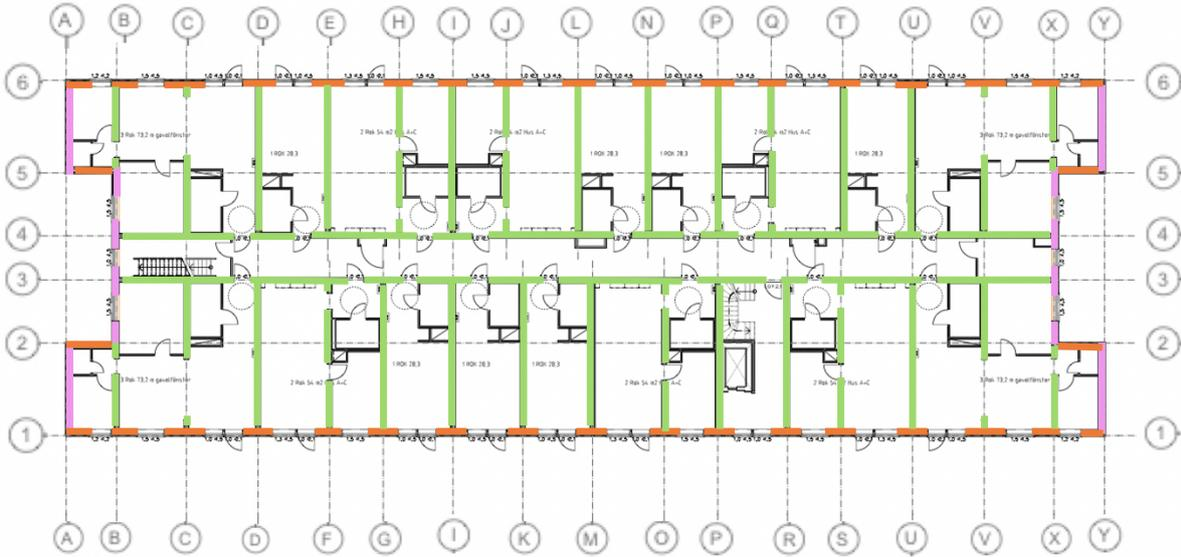
Figure 4.4: The materials of the different walls. Orange = OSB, Pink = OSB and Fibre gypsum, Green = Fibre gypsum.
