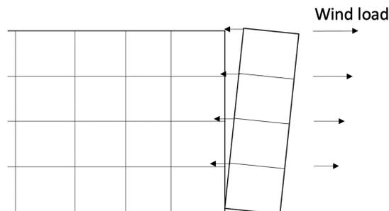
Figure 3.3: Illustration of the outermost modules. View from the long side of the building.
