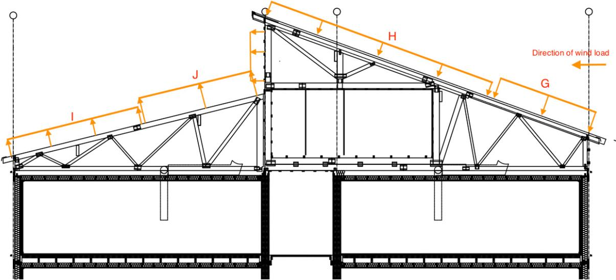
Figure B.7: Worst case for pressure coefficients when the wind load acts on wall 1.
