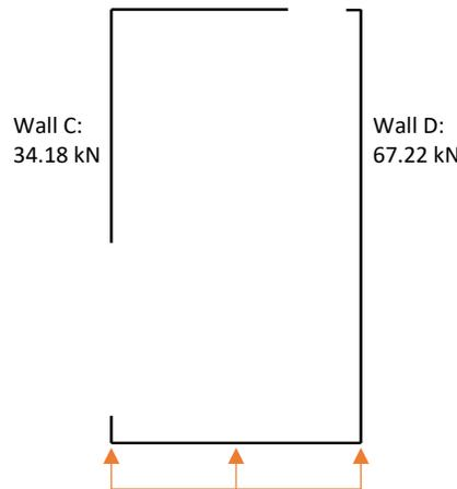
Figure 4.6: Example of how the wind load is divided according to the capacity of the walls.
