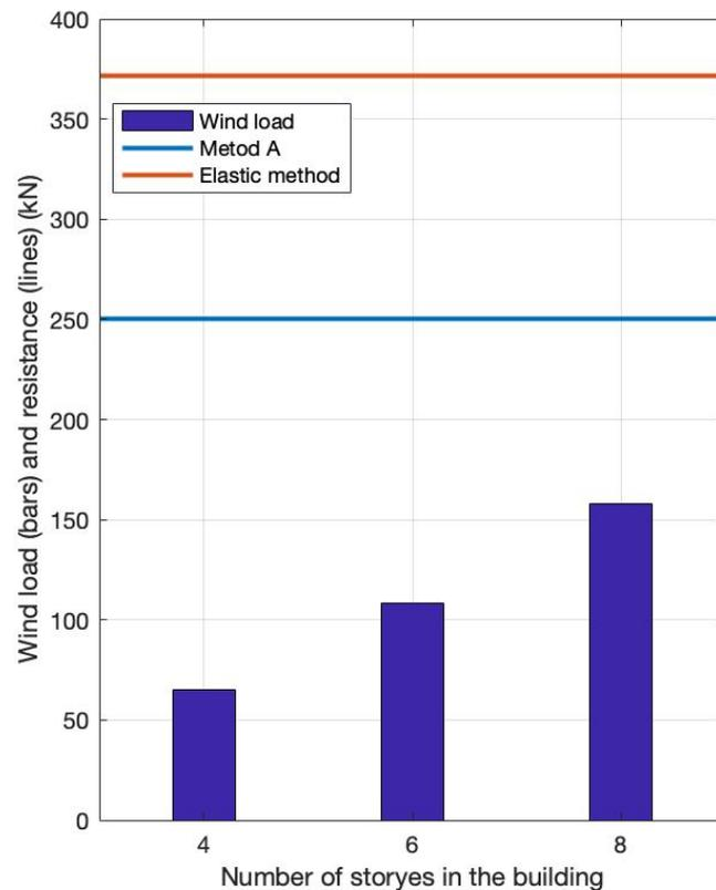
Figure 5.2: The wind load for the three different heights of buildings acting on wall 1 together with the design capacity of the wall according to both methods. Wind on wall A or Y.
