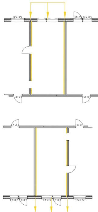
Figure A.12: How the modules in the two structures carry the wind load, when the wind load acts on one of the long sides of the building.
