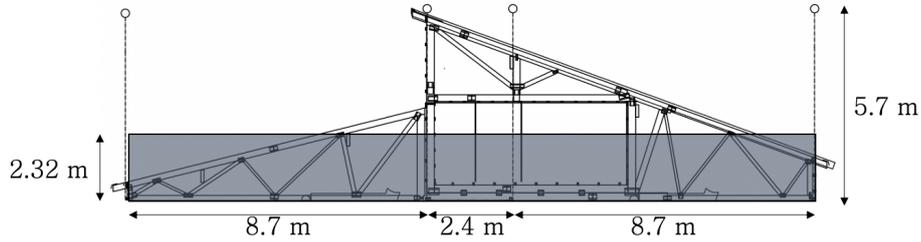
Figure B.9: Equivalent height of triangular area of influence.
