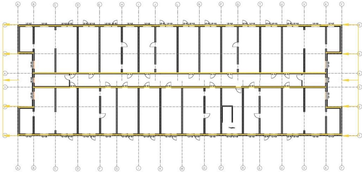
Figure 4.1: Stabilising walls if wind load acts on the short side of the building.
