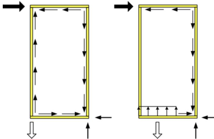
Figure 3.12: Force displacement for plastic calculation model. Complete anchoring of leading stud (left) and incomplete anchoring of leading stud but anchoring of bottom rail (right) (Källsner & Girhammar, 2008). Used with permission.
