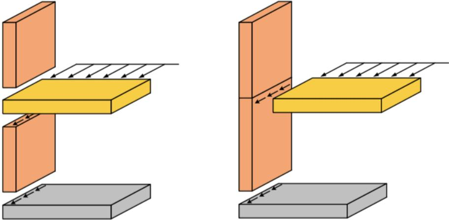
Figure 3.8: How the horizontal loads are carried from the floor to the walls with either supported floor (left) or suspended floor (right) (Källsner & Girhammar, 2008). Used with permission.
