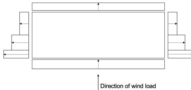
Figure 3.2: Illustration of how the wind load, acting on one of the long sides, is affecting the building. View from a above.
