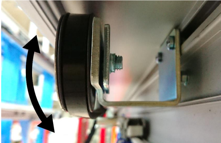
Figure 12 Rocking motion due to lack of wall support
