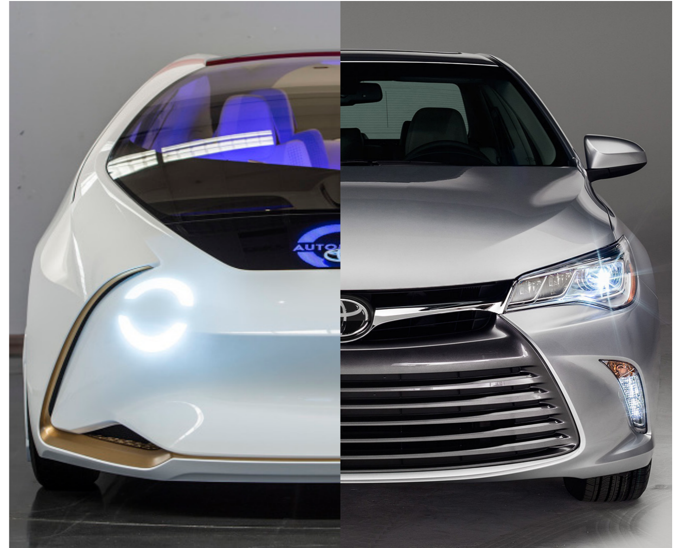
Toyota's 2017 concept car, Concept-i, and the 2015 Toyota Camry Xle. Concept-i's headlights are hidden behind the paint, and can wink as their owner approaches.
