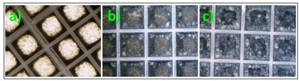
Figure 18. Biofilm on Z-1000 carriers in RMIX. a) day 141. b) day 169 and c) day 232 of operation. Inner dimensions of cells are approximately 2x2 mm.
