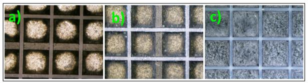
Figure 16. Biofilm on Z-1000 carriers in R1000. a) day 141. b) day 169 and c) day 232 of operation. Inner dimensions of cells are approximately 2x2 mm.
