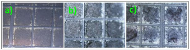
Figure 15. Biofilm on Z-200 carriers in R200. a) day 141. b) day 169 and c) day 232 of operation. Inner dimensions of cells are approximately 2.5x2.5 mm.
