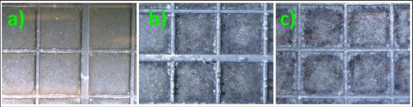
**Figure 17.** Biofilm on Z-200 carriers in RMIX. a) day 141. b) day 169 and c) day 232 of operation. Inner dimensions of cells are approximately 2.5x2.5 mm.
