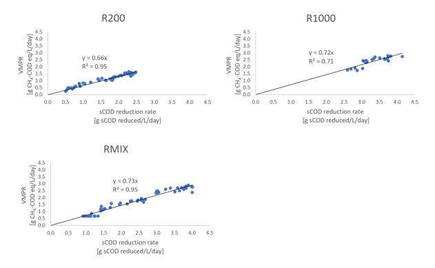
**Figure 13.** Volumetric methane production rate (VMPR) as a function of sCOD removal rate with linear regression forced through the origin.
