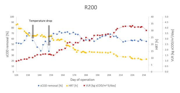
Figure 5. sCOD [%], HRT [h] and VLR [kg sCOD/m3/day] for R200 (containing Z-200 carriers).
