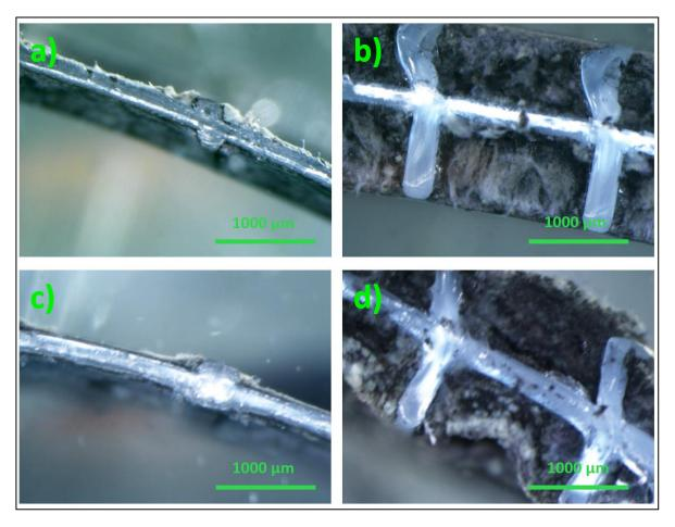
**Figure 19.** Cross section of carriers with biomass at day 232 of operation. a) Z-200 from R200, b) Z-1000 from R1000, c) Z-200 from RMIX and d) Z-1000 from RMIX.
