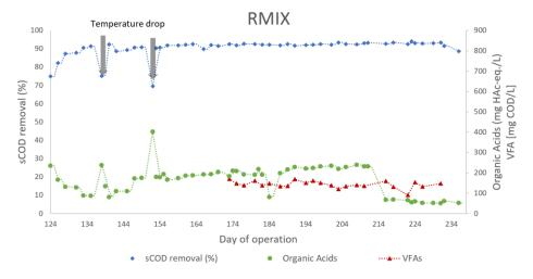
Figure 10. sCOD removal [%], Organic acid [mg HAc-eq./L] and VFA levels [mg COD/L] in RMIX. Due to complications with the GC apparatus, VFA results could only be obtained between day 173-231 of reactor operation.
