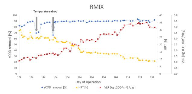
Figure 7. sCOD [%], HRT [h] and VLR [kg sCOD/m3/day] for RMIX (containing Z-200 and Z-1000 carriers).
