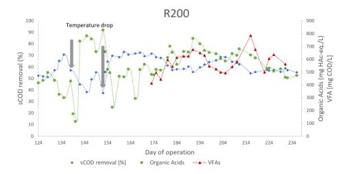
Figure 8. sCOD removal [%], Organic acid [mg HAc-eq./L] and VFA levels [mg COD/L] in R200. Due to complications with the GC apparatus, VFA results could only be obtained between day 173-231 of reactor operation.
