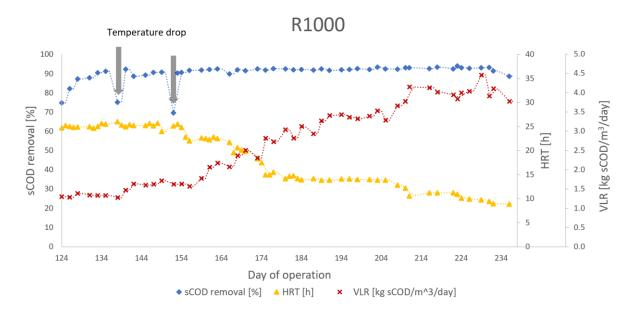
Figure 6. sCOD [%], HRT [h] and VLR [kg sCOD/m3/day] for R1000 (containing Z-1000 carriers).
