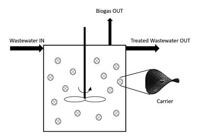
Figure 2. Schematic view of an AnMBBR and an example of a carrier type (the AnoxK<sup>TM</sup> carrier).
