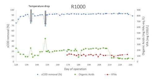
Figure 9. sCOD removal [%], Organic acid [mg HAc-eq./L] and VFA levels [mg COD/L] in R1000. Due to complications with the GC apparatus, VFA results could only be obtained between day 173-231 of reactor operation.
