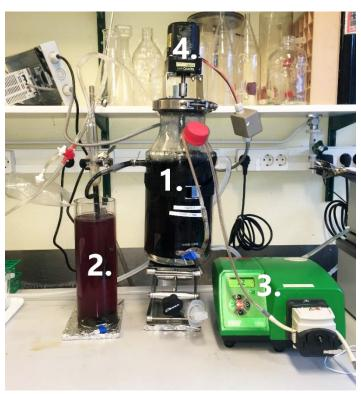
Figure 4. Reactor set-up showing one of the reactors (1) and its effluent trap with overflow (2), feed pump (3) and mechanical stirrer (4).
