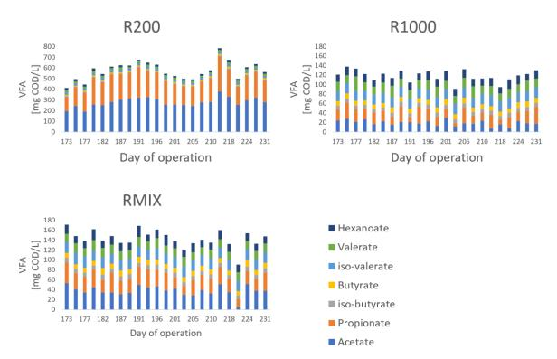
**Figure 11.** VFA concentrations [mg COD/L] in R200, R1000 and RMIX between day 173 and 231. Note the difference in x-axis interval between the reactors. Due to complications with the GC apparatus, VFA results could only be obtained between day 173-231 of reactor operation.
