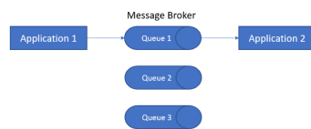
Figure 3.7: A figure showing a publisher sending data to a queue with one consumer
