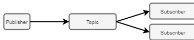
Figure 3.2: Image showing a single publisher sending a message to two separate subscribers
