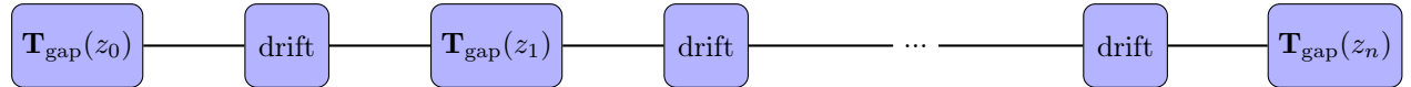
Figure 7: The figure shows how one RF cavity can be approximated by a finite number of thin gaps with drift spaces in between.
