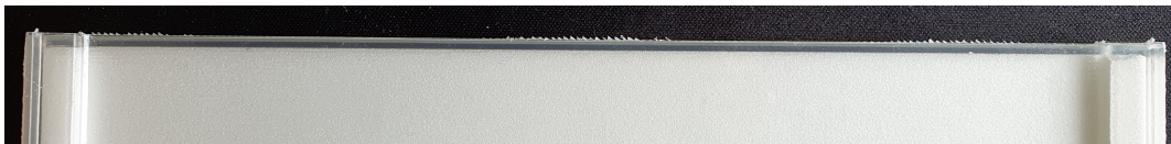
Figure 5.17: Tool sample 006. Total engagement time 684,2 m
