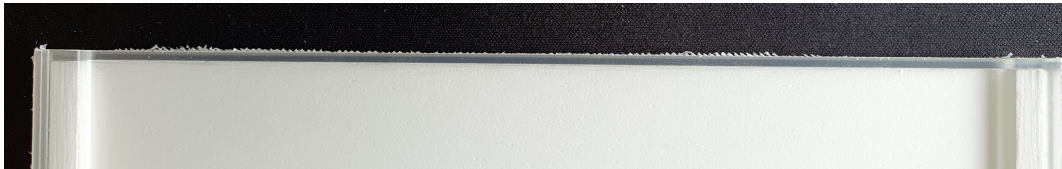
Figure 5.15: Tool sample 004. Total engagement time 665,3 m
