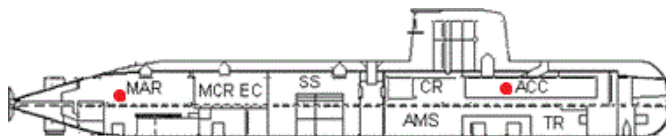
Figure 1: The spots of the two measurement sites in a cross-sectional view of the Gotland Submarine [27].
