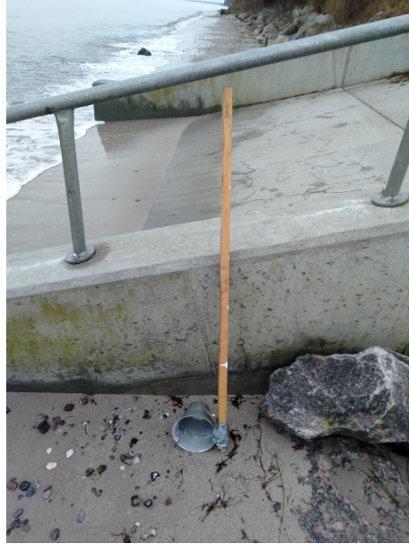
Figure 4.3: Device used to collect nearshore samples, i.e. in the swash zone and at water depth 0.6 m and 1.0 m. Photo: Anna Adell, 2020.
