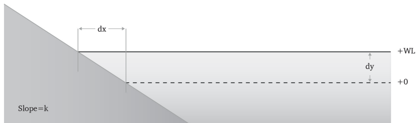
Figure 6.4: Schematic image showing the slope geometry.
