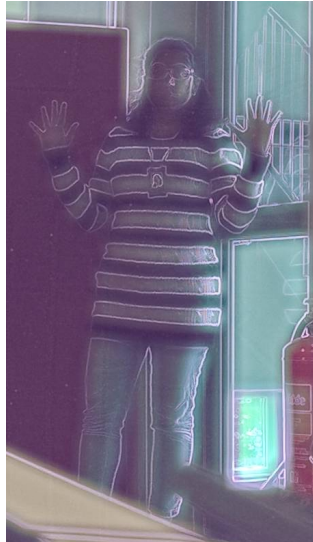
Figure 7.4: Image that is using one Sobel operator per color channel and uses the maximum to calculate the alpha channel.
