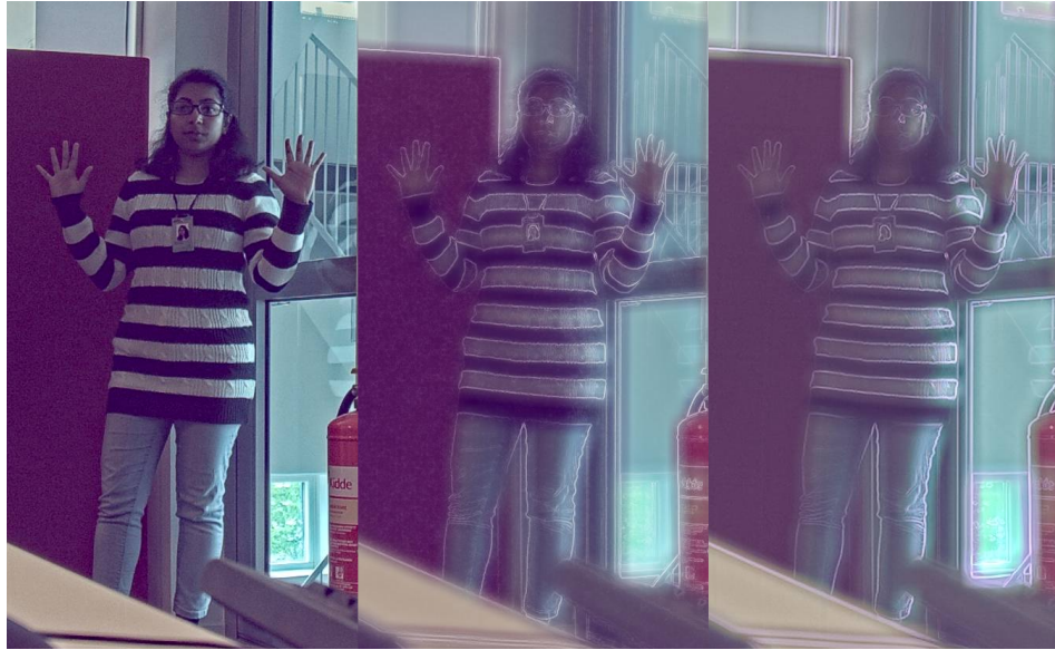
Figure 5.10: RGB images where the left image is without the transformation, the middle one with the reference algorithm applied to it and the right image have gone through the FPGA implementation and the IPP.
