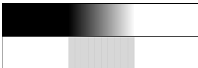
Figure 2.3: The top field is how a more realistic edge looks. The lower is its gradient. It generally have a gradual transition between two mono-colored fields next to each other.
