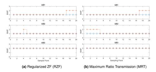
Figure 6.12: Simulation 2B: UEs BWP switching
