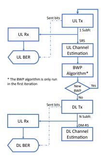
Figure 4.6: Experiment 3 flow.
