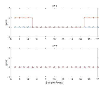
Figure 6.7: Simulation 1B: UEs BWP switching.
