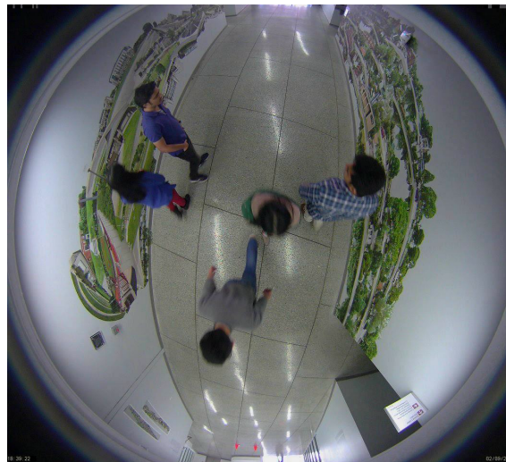
Figure 1.4: A fisheye image captured with top-view perspective, one person is captured almost from straight above. Image from [1].
