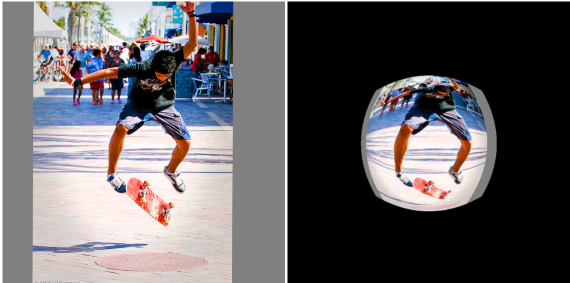
(a) An example image taken from COCO 2014 (b) Same image as in Fig. 6.2a but transformed to resemble a fisheye image.
