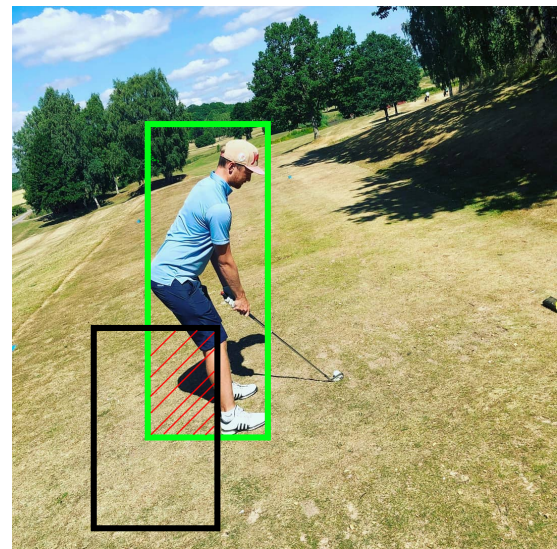
(b) A false positive prediction. The predicted black bounding box overlaps the green ground truth with IoU \leq 0.5 . The striped part is the area of intersection.
