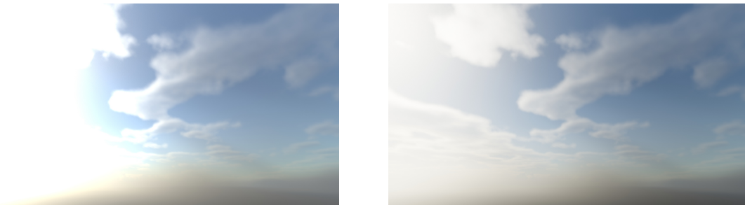
Figure 2.6: The difference between just clamping colour intensities to the low dynamic range (left) and applying the ACES tone mapping operator (right).
