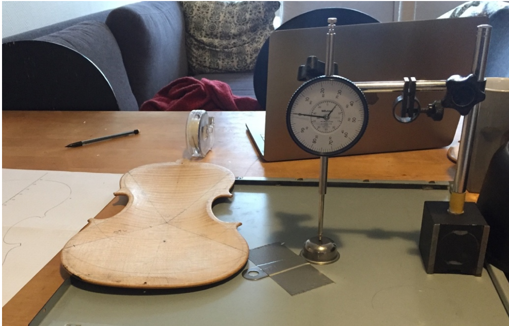
Figure 2.9: Dial indicator setup used to measure the thickness of the plates.
