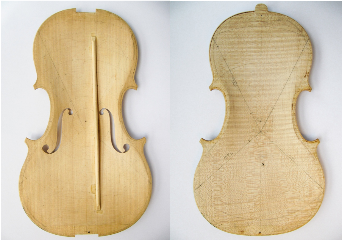
Figure 2.7: A circular coordinate system is used when determining the thickness of the plates.
