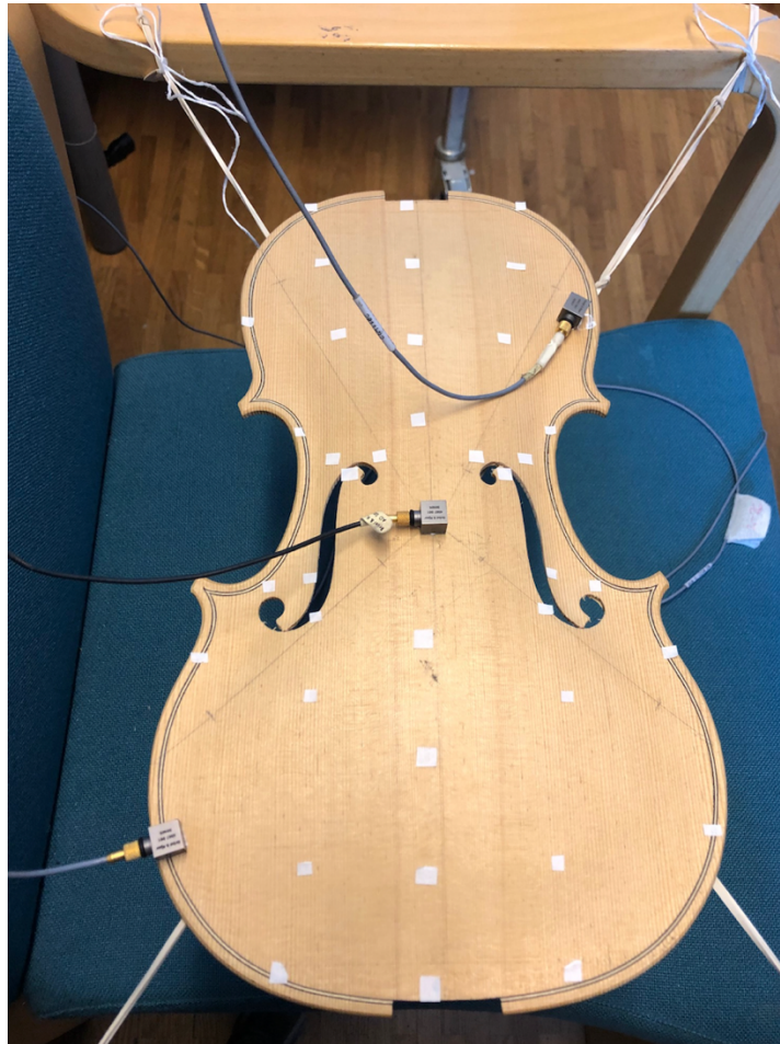
Figure 4.3: Experimental setup for the top plate. Three accelerometers are used. Two are placed close to the corners and the third is placed in the center of the plate to cover all of the first five modes of vibration. The white squares mark the position of the hammer hits.
