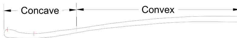
Figure 2.5: Cross-section of one of the plates. The concave shape turns into a convex shape close to the outline.
