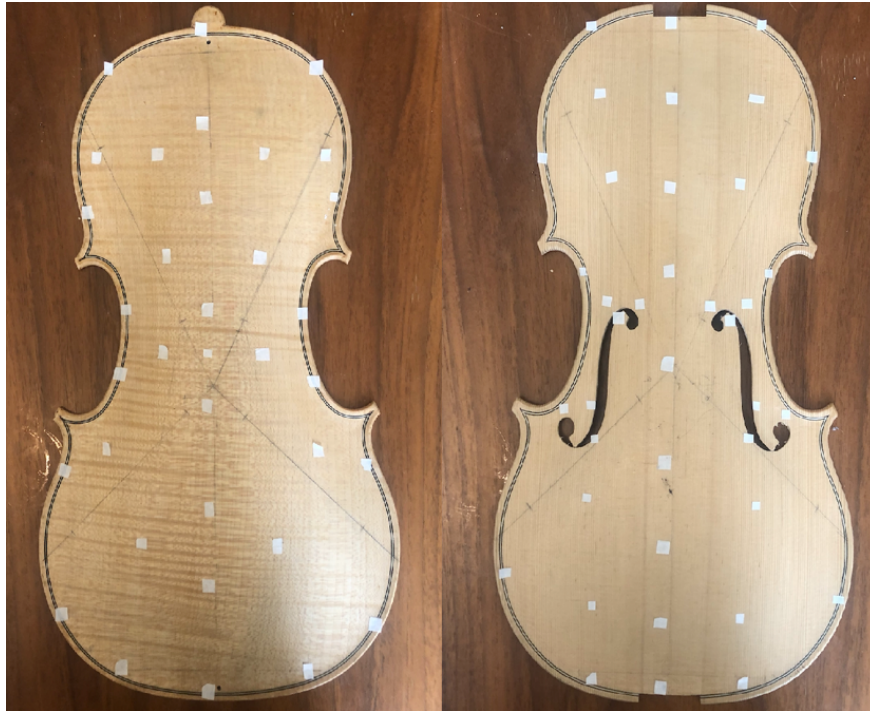
Figure 4.2: The coordinates of every node from the test geometry is transferred to the plates. The position is marked using a piece of tape.
