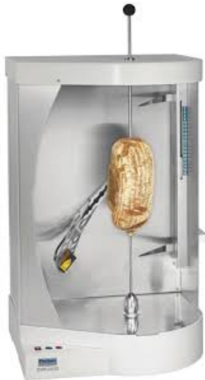
Figure 9. A Perten BVM volume analysis machine (Anderson, Purhagen & Bason, 2014).
