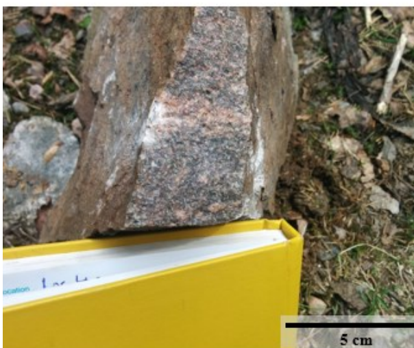
Figure 13. Sample 4g-i is a medium-grained granitic gneiss consisting of plagioclase, quartz and feldspar with abundant biotite.
